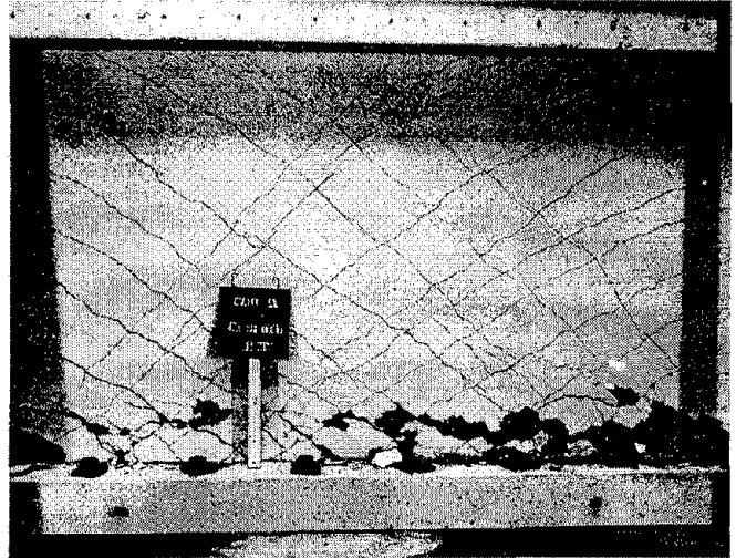
Splitting and Crushing of Concrete at Base of Wall
