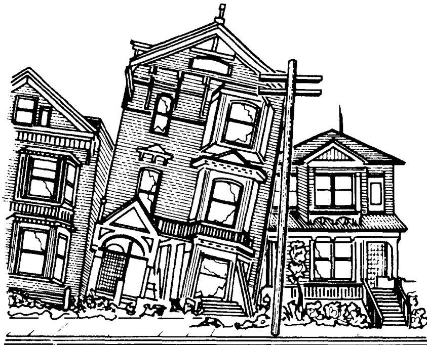
Liquefaction of soil can cause buildings to slump and sometimes to collapse entirely.
