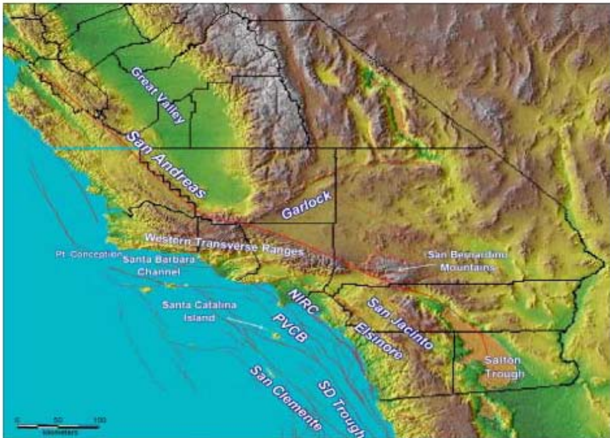
Figure 1. Map showing major faults of the southern California region. Northwest-trending faults are right-slip in character. The “big bend” of the San Andreas fault curves from the Salton Trough to the Great Valley. Major offshore faults include the Newport-Inglewood-Rose Canyon (NIRC), Palos Verdes - Coronado Bank (PVCB), San Diego Trough, and San Clemente. (Shaded relief base map from NOAA State DEM).
