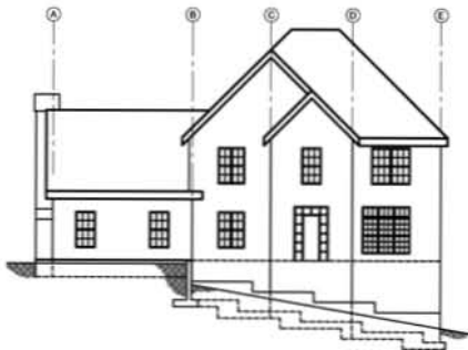
Figure A-3 Hillside base.
