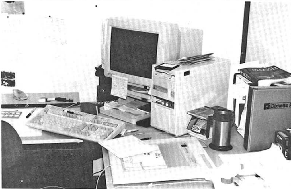
Unsecured computers may fall and suffer damage Photo Credit: Wiss, Janney, Elstner Associates, Inc.
