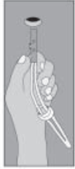
DRILL HOLE. HOLD TOGGLE FLAT ALONGSIDE PLASTIC STRAPS, SLIDE THROUGH HOLE.
