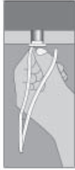
PLACE THUMB BETWEEN PLASTIC STRAPS. PUSH SIDE TO SIDE, SNAPPING OFF STRAPS FLUSH WITH WALL.
