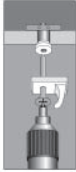
INSERT BOLT THROUGH ITEM TO BE ATTACHED AND TIGHTEN UNTIL FLUSH WITH FIXTURE. MINIMUM CLEARANCE BEHIND WALL: 1-7/8" (48MM).
