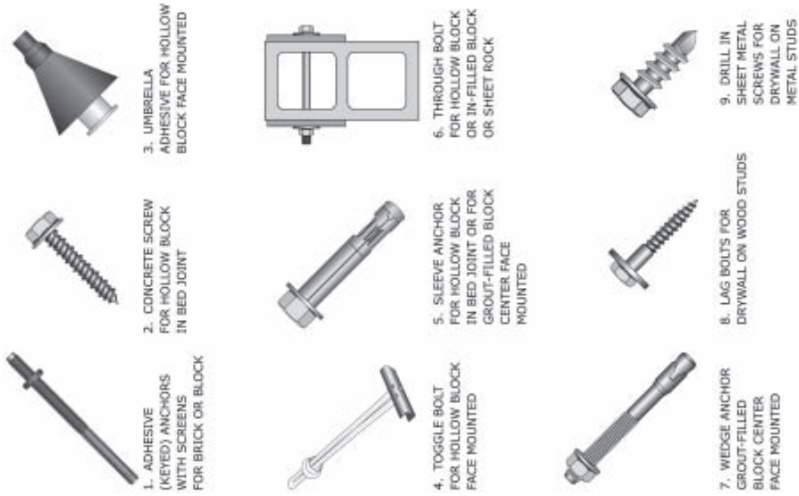
Figure 141: Types of masonry and drywall anchors.
