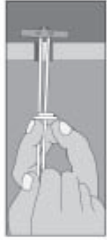
WITH ONE HAND, PULL RING SO METAL CHANNEL RESTS FLUSH BEHIND WALL. SLIDE PLASTIC CAP ALONG STRAPS WITH OTHER HAND UNTIL FLANGE OF CAP IS FLUSH WITH WALL.
