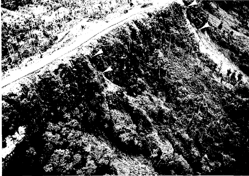
FIGURE 5.3 Landslides (largest examples are indicated by arrows) in residual soils at the top of the N valley wall of the Quijos River between El Chaco and the confluence of the Quijos and Salado Rivers. Because slide-resistant sedimentary bedrock (light-colored outcrop at the lower left) is close to the surface, these slides/avalanches are shallow and generally limited to existing gullies. Although the slides endangered the Trans-Ecuadorian pipeline and highway (angling across top of photo above the landslides), they caused little actual damage because they were so shallow.
