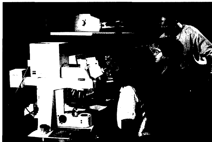
Drs. Lipin Sung, Mary McKnight and Geoffrey Frohnsdorff view a confocal microscopic image of an optical slice through the thickness of a coating. The confocal microscope has an optical resolution down to 200 nm and is a major research tool in assessing the microstructural properties of coatings.
