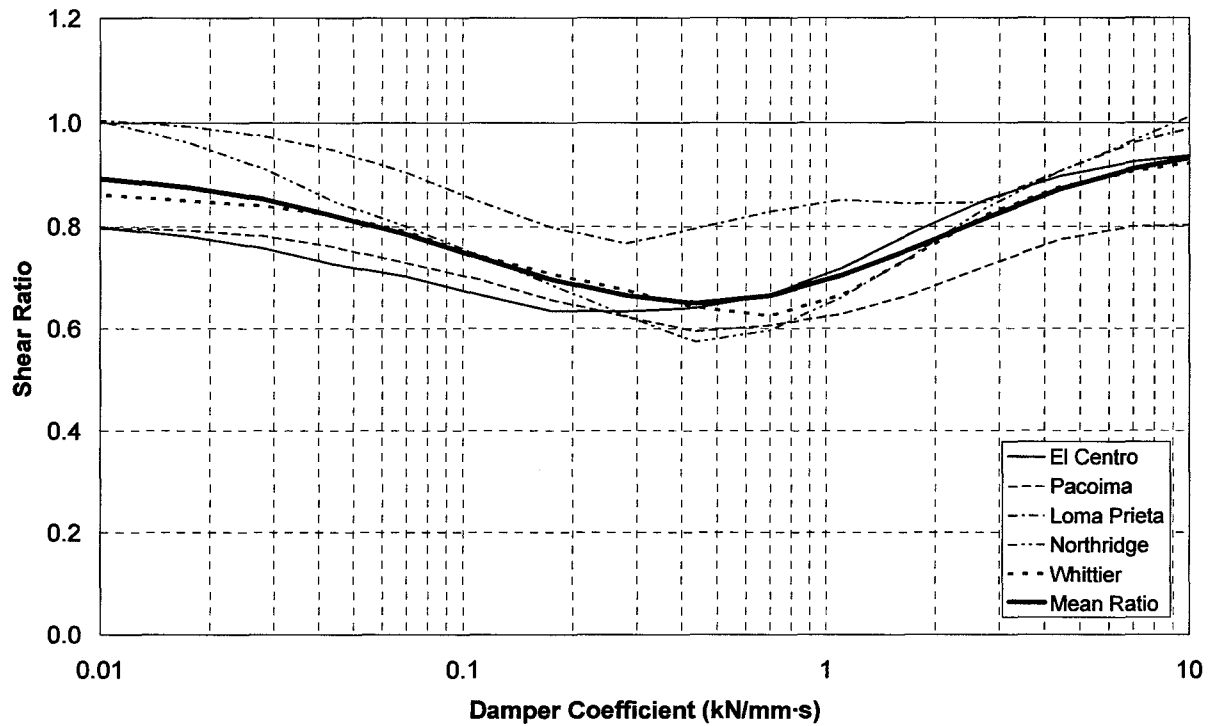
Figure 4.31 Shear connector stress ratio with VE dampers connected to abutments.
