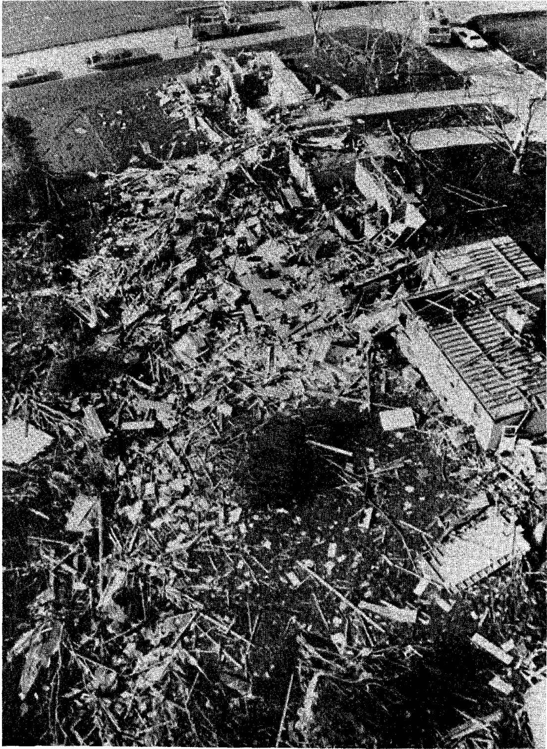
Figure 3. Debris pattern indicative of strong vortex motion (courtesy R. Paskach, Omaha World-Herald).
