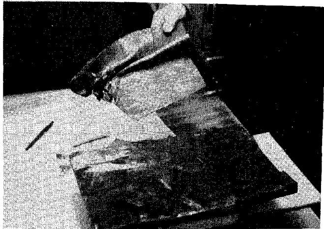
Figure 29 Incienso Dislodged Neoprene Bearing Pad
