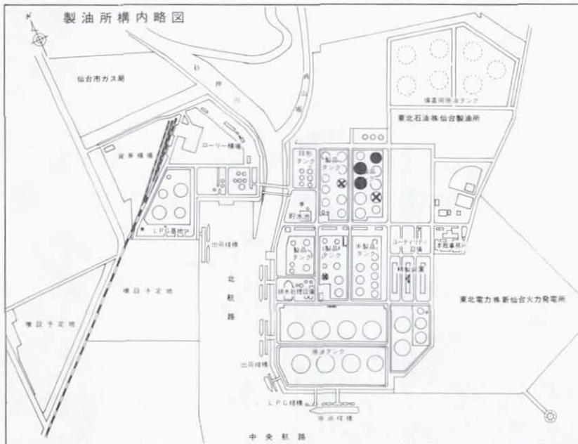
Figure 6.40 Plan of the Sendai Refinery, Tohoku Oil Company, Ltd. Tanks are shown as circles in the plan. The circles that represent the three failed TC tanks have been blackened; ones that represent the three other damaged tanks are marked with an X. The refinery structures are located to the right of the tank farms.
