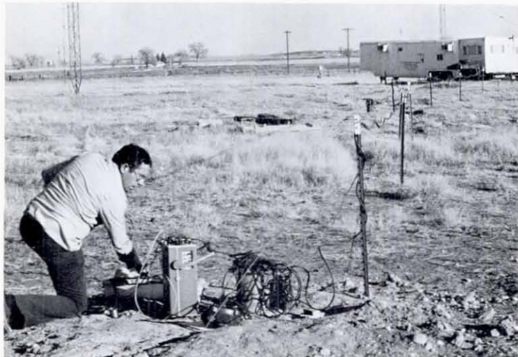
On a tiltmeter testing site near Erie, Colo., Levine troubleshoots an electrical problem with one of the tiltmeters buried 30 meters beneath this prairie land. A microcomputer, housed in a trailer in the background, takes data from the tiltmeters and sends it to the laboratory in Boulder.
