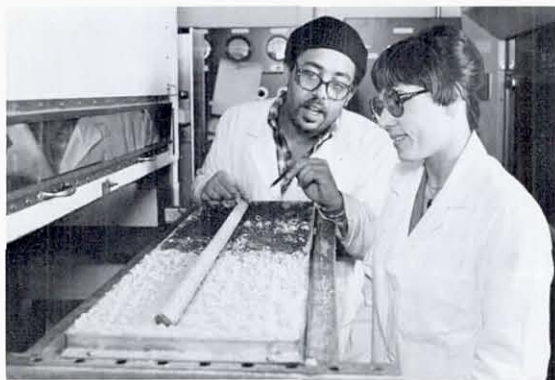
NVLAP project leader Diana Kirkpatrick and engineering technician Thomas Prather measure the distance burned in a radiant panel test for flammability of loose-fill cellulosic insulation.
