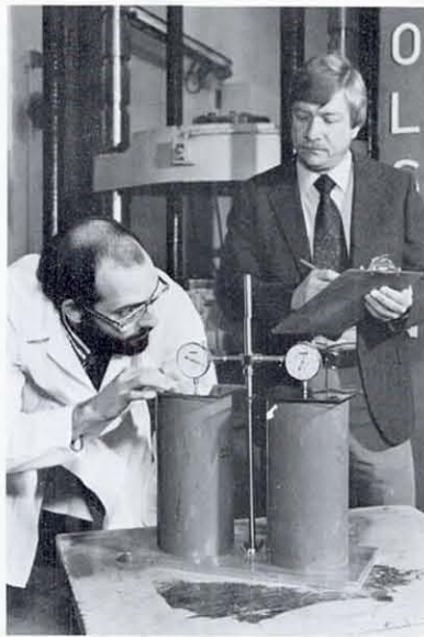
Rick Seifarth (left), an NBS Cement and Concrete Reference Laboratory inspector, and Bob Gladhill, a NVLAP project leader for the concrete LAP, verify the dimensional stability of two concrete cylinder molds.
