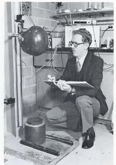
Douglas Thomas, project leader for the proposed athletic equipment LAP, inspects a monorail system used to measure the impact resistance of football helmets.
