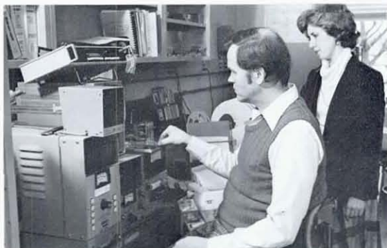
Thomas Hobbs, chief of health physics in the Occupational Health and Safety Division, takes a reading of a thermoluminescent radiation detector for personnel dosimeters. Observing the procedure is Margaret Federline, project leader of a LAP for processors of personnel dosimeters.
