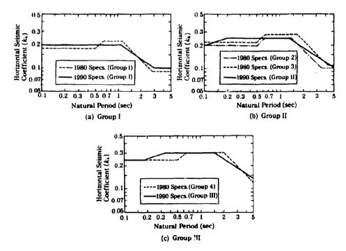
Fig.3 Comparison of Scismic Coefficient between 1980 and 1990 Specifications
