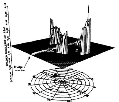
Figure 11. Summary Plot Of Wind Speeds And Maximum Bridge Accelerations.
