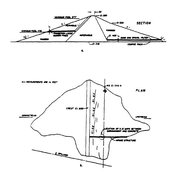
Fig. 7. Newell Dam. a. Typical section. b. Plan of dam showing longitudinal cracks along upper upstream face.
