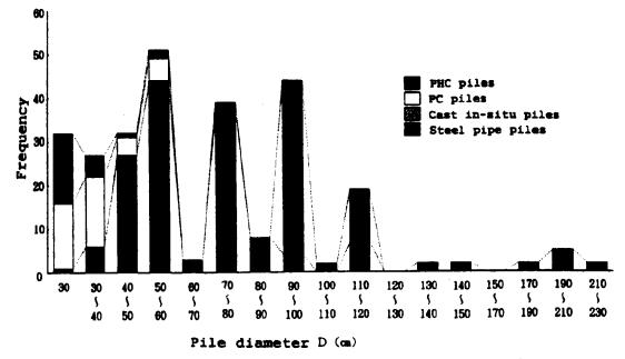
Figure 1. Frequency distribution of pile diameter
