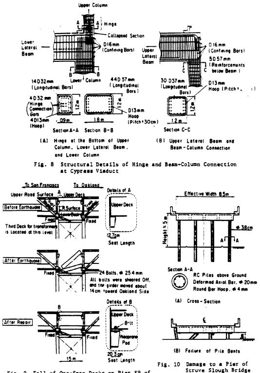
Fig. 9 Fall of One-Span Decks on Pier E9 of Bay Bridge and Outline of Its Repair
