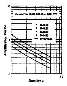
Figure 4. Amplification Factors for PSV<sub>mer</sub> in the Velocity Region [from Wu (1987)]
