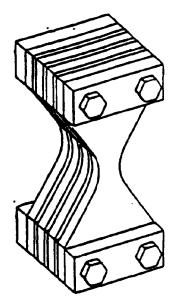
Figure 15. Added Damping and Stiffness (ADAS) Steel Plate Damper [from Bergman (1987)]
