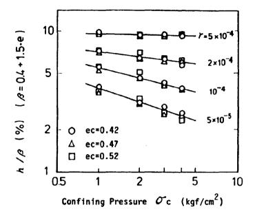
Fig. 7 h/ $\beta$  versus Confining Pressure  $\sigma_c$  (CTSS)
