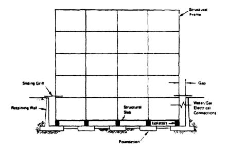
Figure 5. Typical layout for base isolated building.
