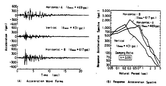
Fig. 2 Acceleration Wave Froms and Response Acceleration Spectra (for Damping Ratio of 5%) Recorded at Corralitos Closest to the Epicenter (from CDMG)
