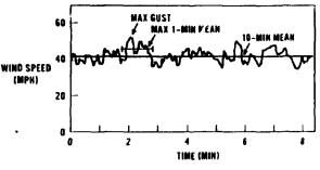
Figure 8 Variation of wind speed at a fixed elevation showing typical averaging time intervals.
