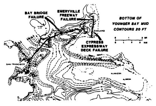
Figure 3. Bottom of younger bay mud with locations of Cypress Expressway deck failure, the Emeryville Preeway failure and the Bay Bridge failure. Contours from Goldman (1969).
