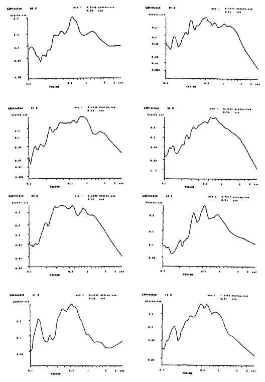
Fig. 6(b) Fourier Spectra of Microtremor in LENINAKAN
