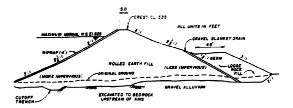
Fig. 6. Elmer J. Chesbro Dam. Typical section.
