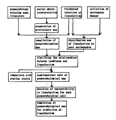
fig.10- A flowchart to compile a geomorphological map for prediction of liquefaction  $\label{eq:complex}$
