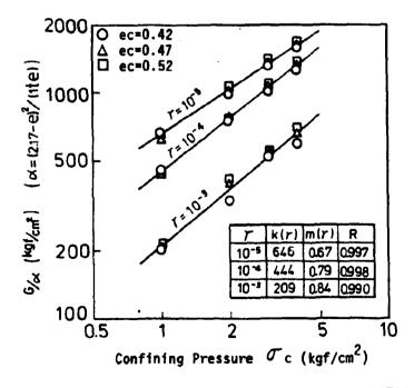
Fig.4 G/ $\alpha$  versus Confining Pressure  $\sigma_{\bullet}$  (CTSS)
