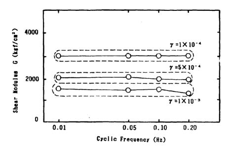
Fig. 9 Shear Modulus G versus Cyclic Frequency (CTSS)
