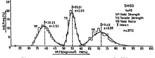
Fig.-2 Histogram of Mechanical Properties for SM50
