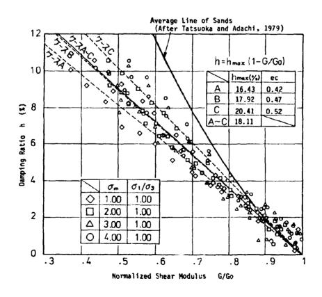
Fig. 10 Damping Ratio versus Normalized Shear Modulus (CTSS)
