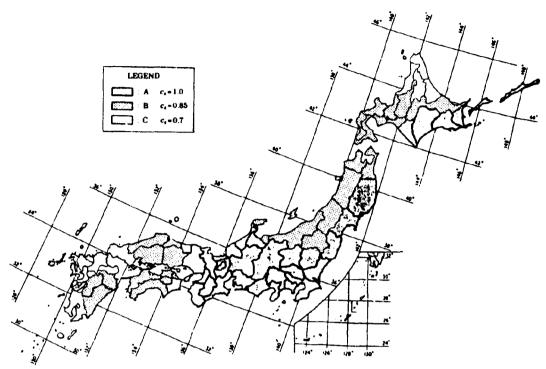
Fig.2 Scismic Zoning Map and Modification Coefficient cz
