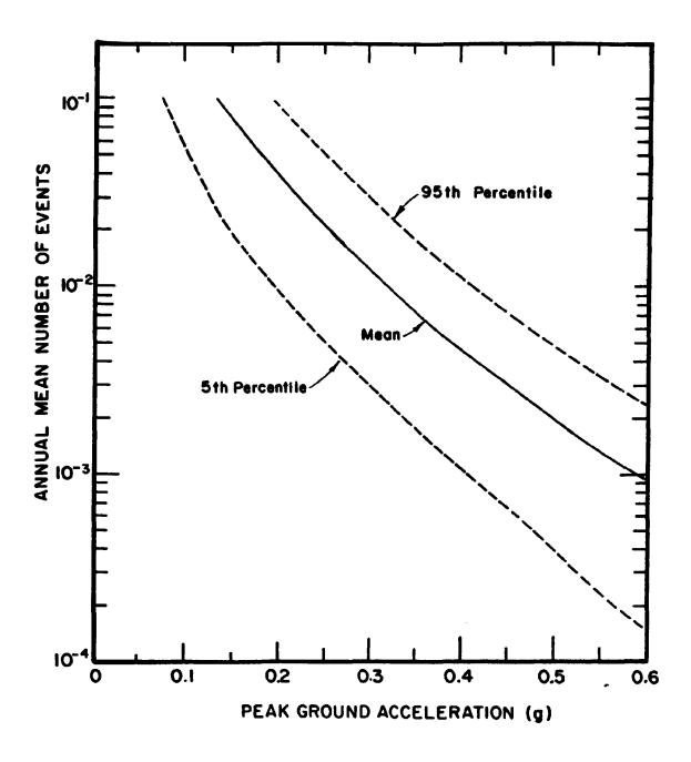
Figure 2a Seismic Hazard Curves for all LLNL site: Peak Ground Acceleration (g).
