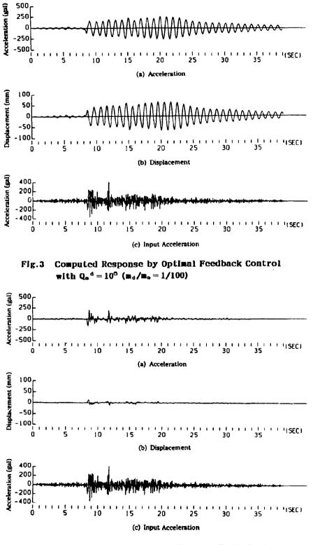
Fig.4 Computed Response by Optimal Feedback Control with  $Q_0^{d} = 10^{10} (m_d/m_0 = 1/100)$
