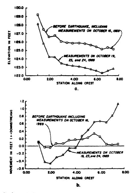
Fig. 3. Austrian Dam. a. Shows cumulative settlement along dam crest just before and after October 17, 1989, earthquake. b. Shows herizontal transverse movements of crest survey points just before and after earthquake.
