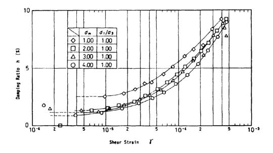
Fig. 2(b) Strain Dependent Curves of Damping Ratio h (CTSS)
