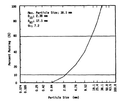
Fig. 1 Grain Size Distribution Curve of Specimen
