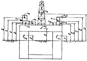
Figure 11 Wind-exposed areas on a model of a floating offshore drilling rig.
