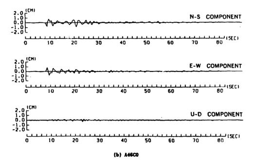
Figure 5 Time History of the Calculated Displacement (A2C0 and A46C0, EQ-28)
