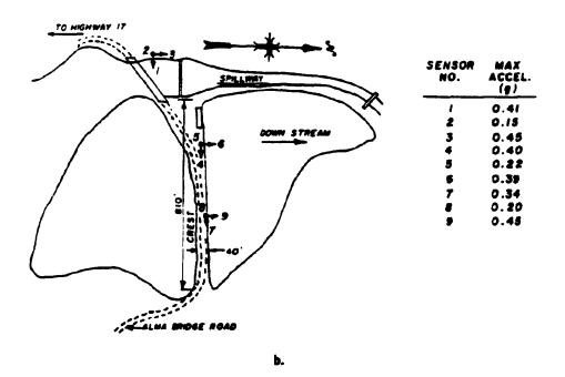
Fig. 8. Laxington Dam. a. Typical section. b. Flan of dam showing location of strong-motion instruments and table of maximum accelerations of strong-motion instruments.
