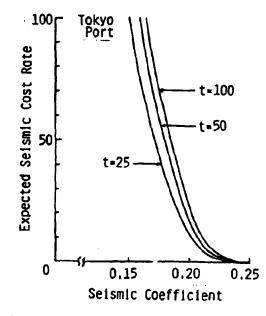
Fig.11 Expected Seismic Cost Rate versus Seismic Coefficient
