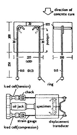
Figure 1: Loading Apparatus for Pull Out Test of Standard hooked Anchorage
