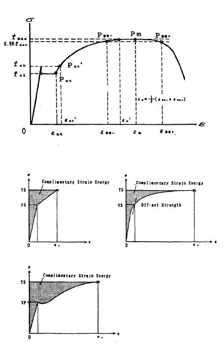
Fig.-8 Shapes of Stress-Strain Curves
