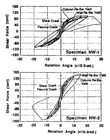
Figure 6: Shear Force vs. Rotation angle Relationship
