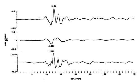
Figure 4. Calculated displacements at Oakland Outer Marbor Wharf (upper), Yerba Buena Island, and their difference (lower), in the 80° direction, approximately in the longitudinal direction of the Bay Bridge.
