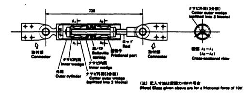
Figure 10. Cylindrical Friction Damper
