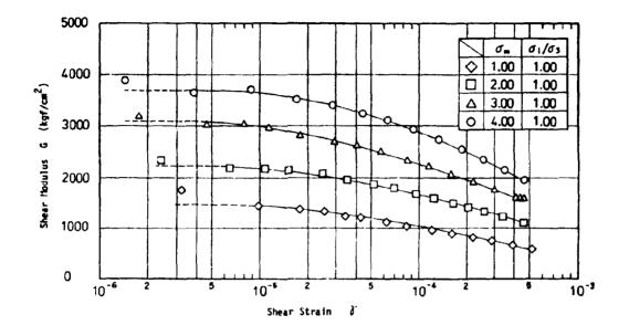
Fig. 2(a) Strain Dependent Curves of Shear Modulus G (CTSS)
