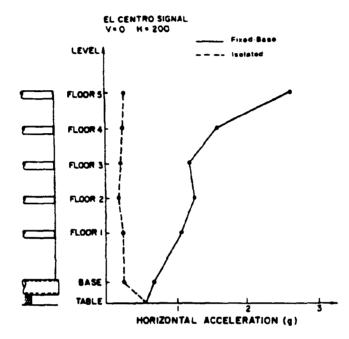
Figure 4. Floor accelerations for five-story, one-third scale model steel frame building loaded by 1940 El Centro earthquake time history with a scaled peak acceleration of 0.55g (after Ref 16).
