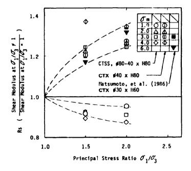
Fig. 8 R, versus Principal Stress Ratio  $\sigma_1/\sigma_3$  (CTSS and CTX)
