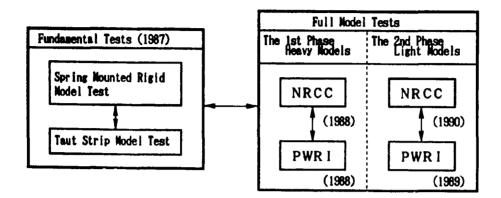
Figure-1 PROGRAM OF COOPERATIVE WIND TUNNEL TEST
