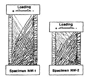
Figure 7: Crack Pattern
