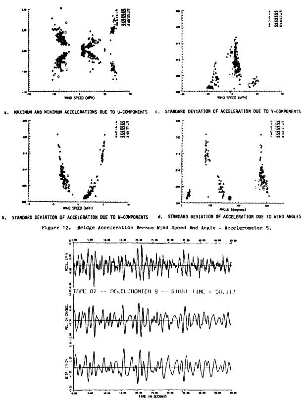
Figure 13. Bridge Acceleration, Velocity, Displacement - Accelerometer 9.
