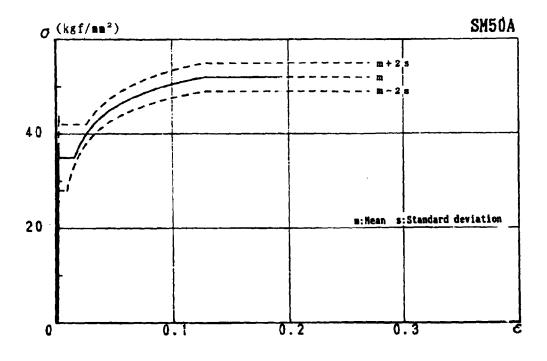
Fig.-10 Standardized Stress-strain Relations for SM50
