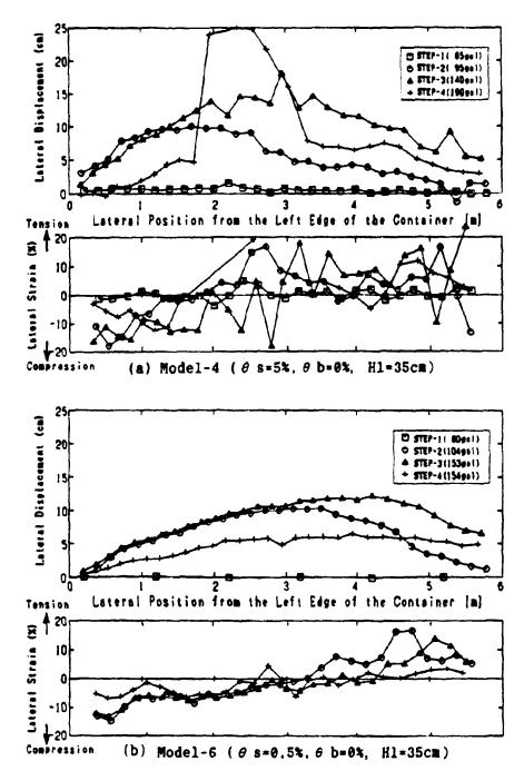
Fig. 2 Lateral Deformation of Ground Surface Resulted from Bench Mark Points
