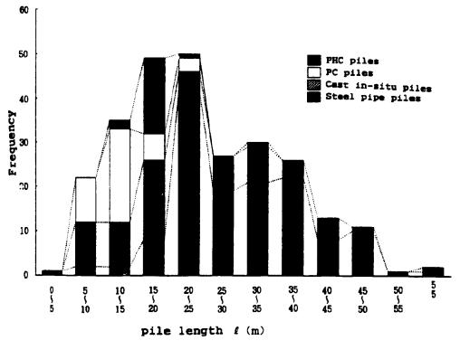
Figure 2. Frequency distribution of pile length
