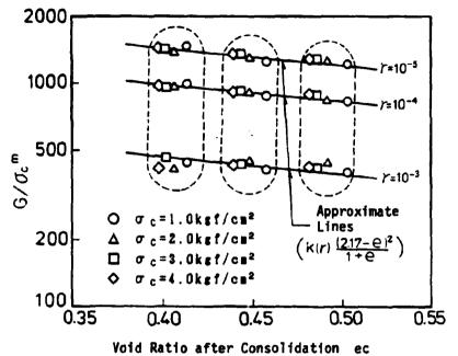
Fig.3 G/0 m versus Void Ratio e. (CTSS)
