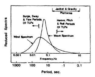
Figure 12 Excitation and frequency ranges of offshore platforms.
