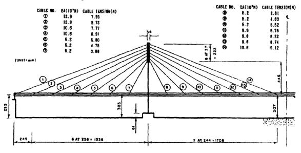
Figure-4 CABLE ARRANGEMENT (NRCC)
