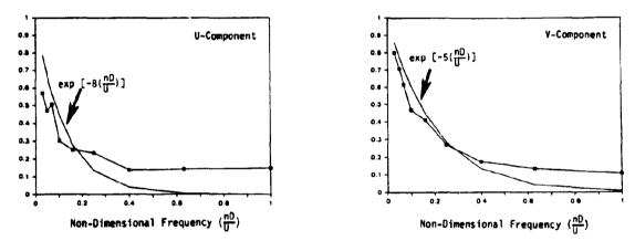
Figure 10. Along-Span Coherency For A 44 mph (20m/s) Perpendicular Wind (80°).
