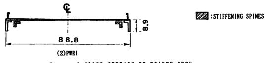
Figure-2 CROSS-SECTION OF BRIDGE DECK
