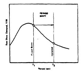
Figure 1. Idealized base shear demand versus period curve.
