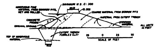
Fig. 9. Vasona Percolation Dam. Typical section.
