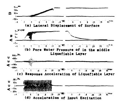
Fig. 4 Relation Between Lateral Displacement of Surface, Pore Water Pressure and Acceleration of Liqueflable Layer (Model-6, Step-2, Section-A)
