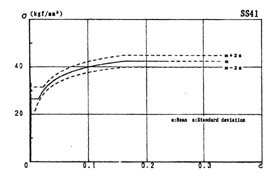
Fig.-9 Standardized Stress-strain Relations for SS41
