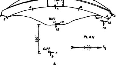
Fig. 12. Lower Crystal Springs Dam. a. Typical section showing locations of strong-motion instruments and table of maximum accelerations during the main event of the October 17, 1989, earthquake. b. Plan of dam showing locations of strong-motion instruments.
