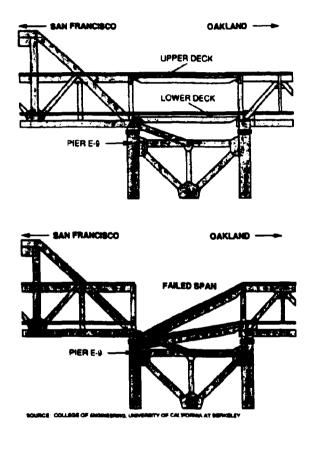
Figure 4: Failure of the Bay Bridge during the Loma Prieta Earthquake
