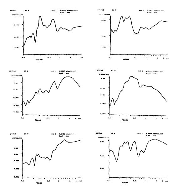
Fig. 9(b) Fourier Spectra of Microtremor in SPITAK
