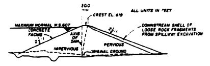
Fig. 4. Almaden Dam. Typical section.
