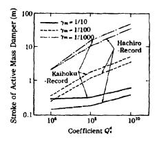
Fig.6 Stroke Required by Optimal Feedback Control
