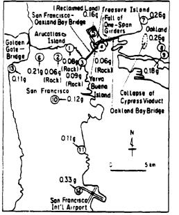
Fig. 3 Distribution of Peak Accelerations on Ground Surfaces and First Floors of Buildings (from USGS and CDMG)
