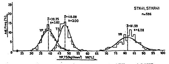
Fig.-3 Histogram of Mechanical Properties for STK41 and STKR41
