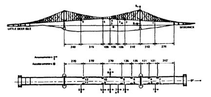
Figure 2. FHWA Instrumentation Layout.
