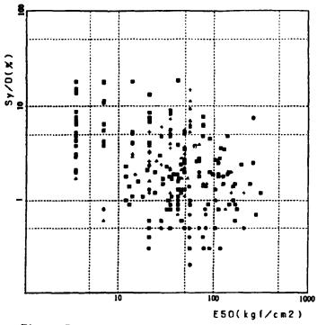
Figure 5. Relation of Sy/D~  $E_{so}$  for all piles
