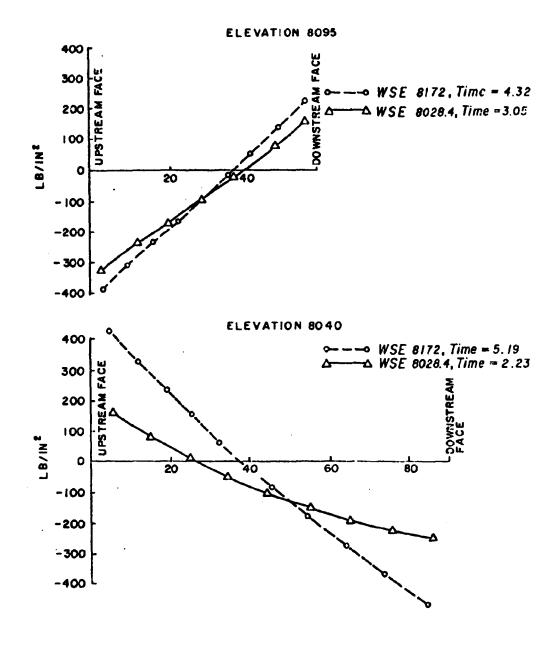
Fig. 9 VERTICAL STRESSES AT MAXIMUM SECTION WATER + DEAD LOAD + MCE
