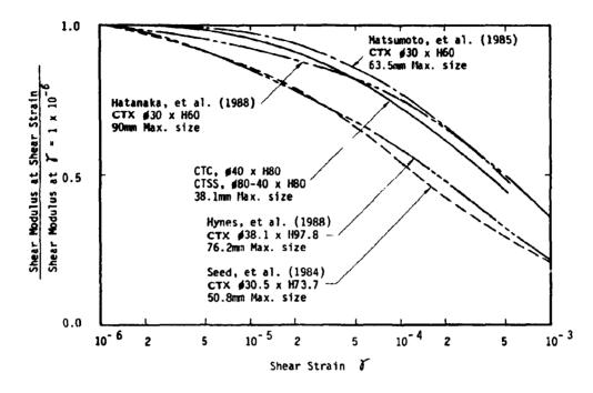
Fig. 11(a) Relationship between Normalized Shear Modulus  $G/G_0$  and Shear Strain  $\gamma$
