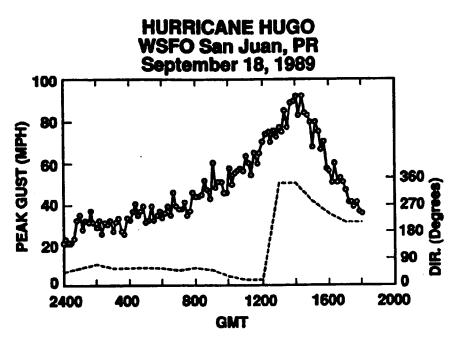
Figure 15a. Time-plot of measured peak gust windspeeds during flurricane HUGO's strongest period at NWS San Juan, P.R. See text for details. Courtesy of R.D. Marshall.
