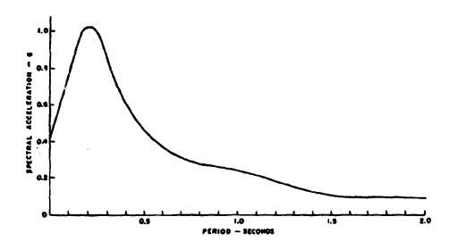
Fig. 2 RESPONSE SPECTRUM M 64 AT 2 KM - 5 % DAMPING
