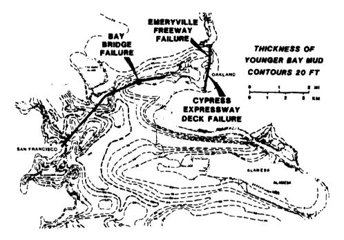
Figure 2. Thickness of the younger bay mud with locations of Cypress Expressway deck failure, the Emeryville Freeway failure and the Hay Bridge failure. Contours are from Goldman (1969).
