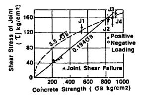
Figure 11: Relationship of Maximum Shear Stress vs. Concrete Strength
