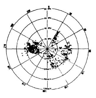
WIND ANGLE VS. RESULTANT WIND VELOCITY TOP OF NORTH TOMER
