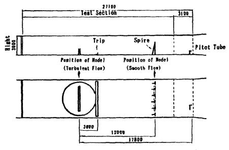
FIGURE-5 ARRANGEMENT OF TURBULENCE GENERATER (PURI)
