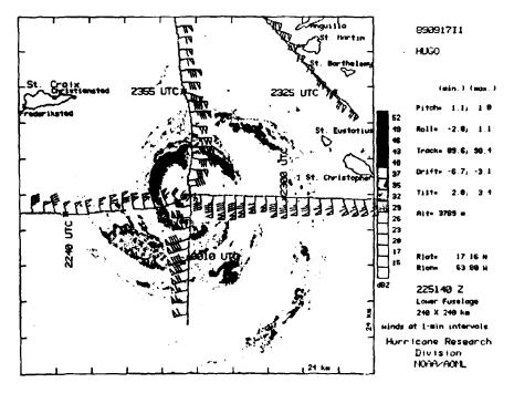
Figure 13a. Composite analysis of radar reflectivities flight track and one-minute sustained winds at 10,000 ft flight altitude of NOAA P-3 aircraft, centered around time 2251 GMT, 9/17/89 as HUGO was nearing St. Croix (upper left). Wind symbol convention is triangle=50kts and ea. full barb=10kts. Courtesy Marks and Powell, HRD.
