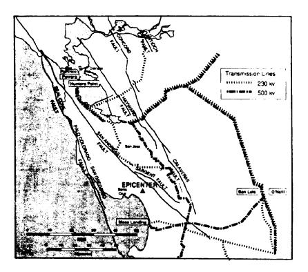
Figure 7: Electric power system in the earthquake-affected areas
