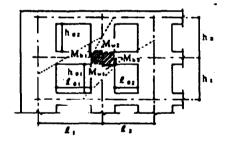
Fig. A 9.5.2 Notation for Design of Bearing Wall-Wall Girder Joint
