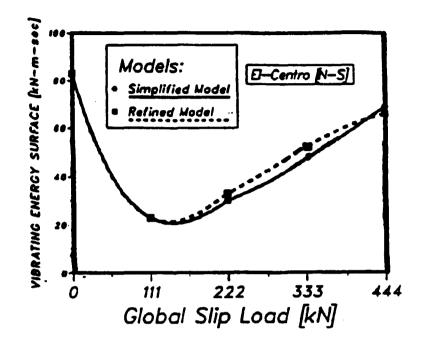
Figure 9. Optimum Slip Load for Friction Damped Braced Frames Subjected to Six Seconds of El C. ntro 1940 Accelerogram [adopted from Univ. of British Columbia]
