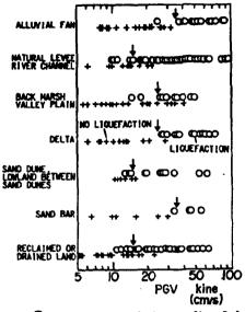
Fig. 8 Peak ground velocity at liquesed and non-liquesed sites on various geomorphological units
