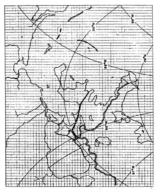
Figure 2b. A transformation of Fig. 2a. onto an image plane. The grid lines intersect as squares. Equally spaced surge values can be printed with a line printer. The projected latitude-Longitude lines are distorted line printer. accordingly.
