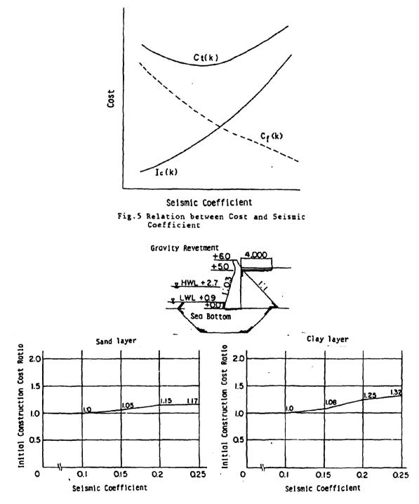
Fig.6 Initial Construction Cost versus Seismic Coefficient (Gravity Revetment)
