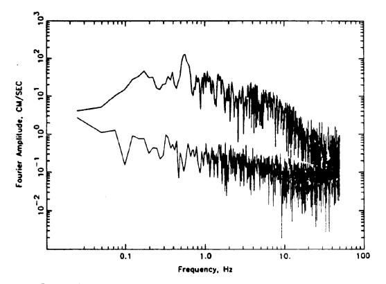
Figure 2. Fourier amplitude spectra of Anderson dam, left abutment, 243° component suppery and a reference trace processed identically (lower); no long-period filter, subtraction of fixed trace, and subtraction of mean.
