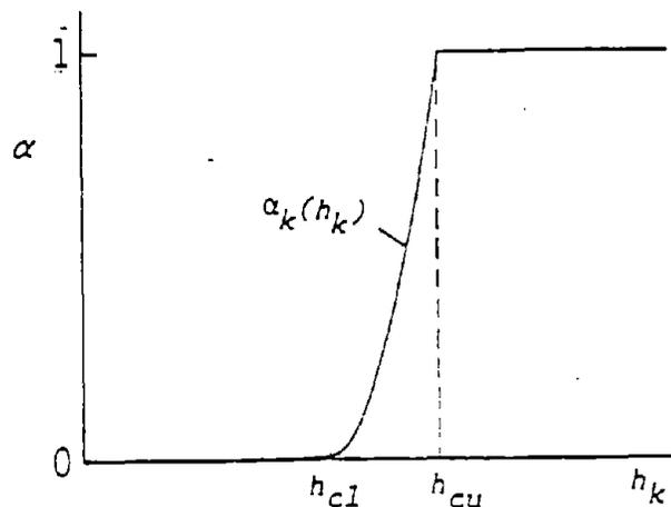
Figure 4. A typical variation of  $\alpha$  with  $h_k$ .
