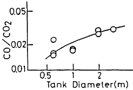
Figure 6 Relationship between CO/CO<sub>2</sub> and tank diameter
