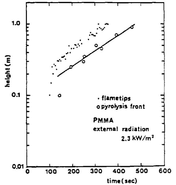
Figure 11 Location of Flametips and Pyrolysis Front
