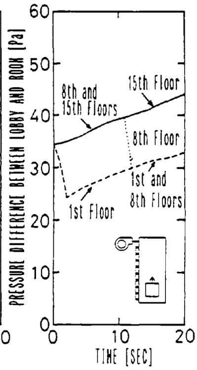
Figure-8. Calculation results when air supply on each of the floors and a cage ascends
