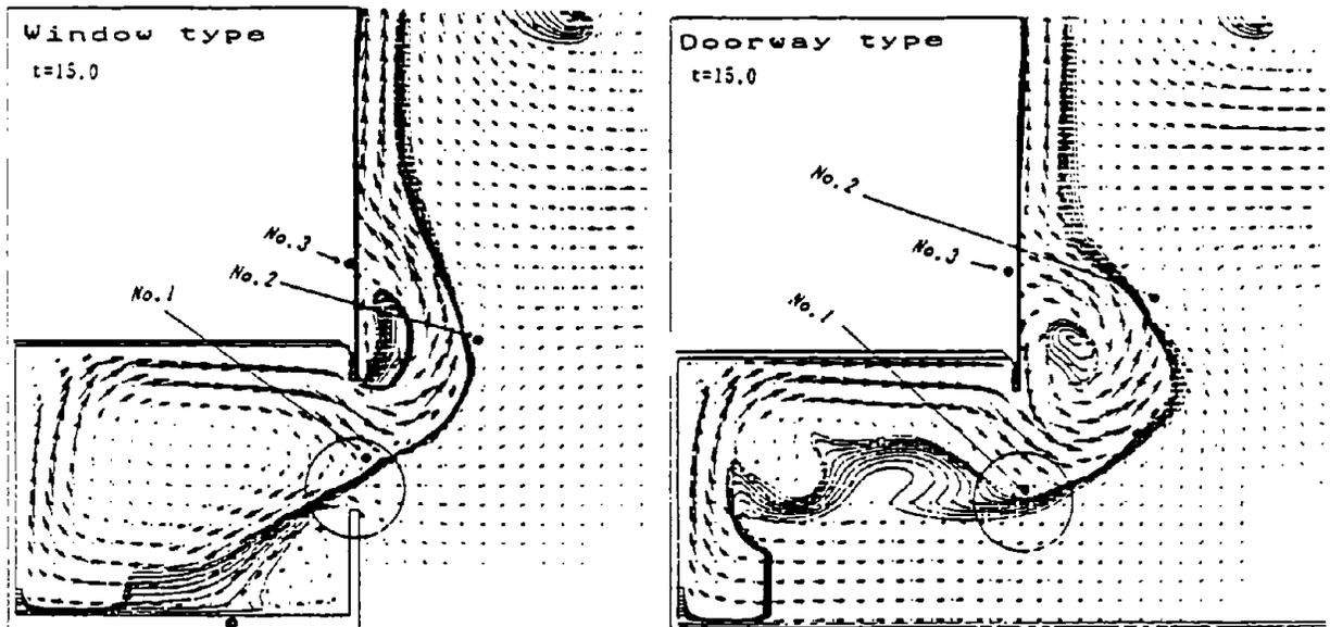
Fig. 1 Calculated flow patterns (previous study<sup>12</sup>) by velocity vector distributions and isothermal lines (isotherms are displayed only in the vicinity of the boundary of hot gas and cool air.)
