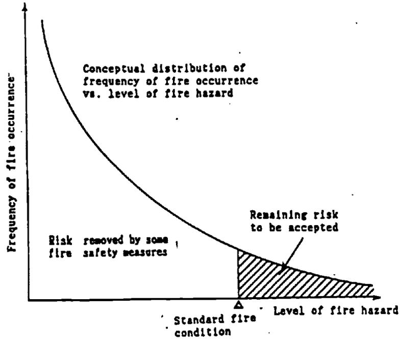
Figure 4. Meaning of standard fire condition
