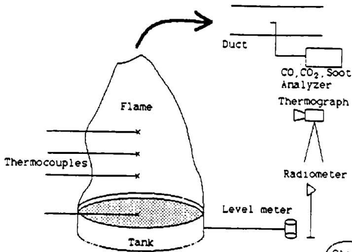
Fig.1 Schematic of experimental set up
