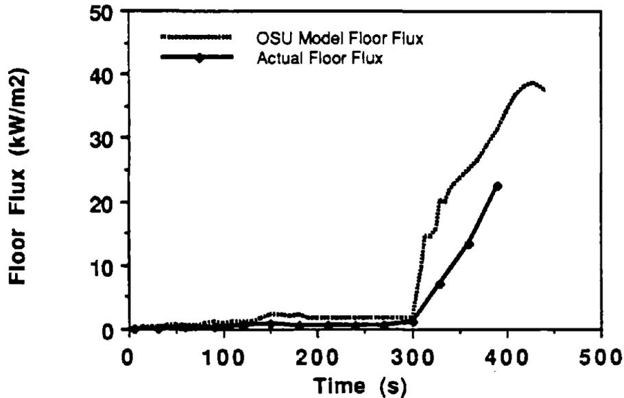
The predicted heat release from the OSU ROOM Model agrees quite well with the actual heat output during the first five minutes of the test. After the propane flow was increased to 160kW the model predicts a slower rate of growth on to flashover than actually occurred. Because there was a delay in the measurement of the heat released from the room, the data has been shifted to
