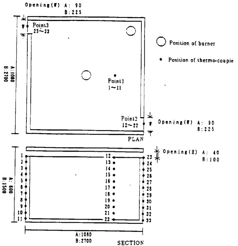
Fig.5 Plan and Section of Models (A:1/25, B:1/10)
