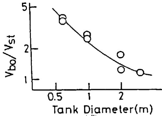
Figure 7 Relationship between V<sub>st</sub>/V<sub>bo</sub> and tank diameter
