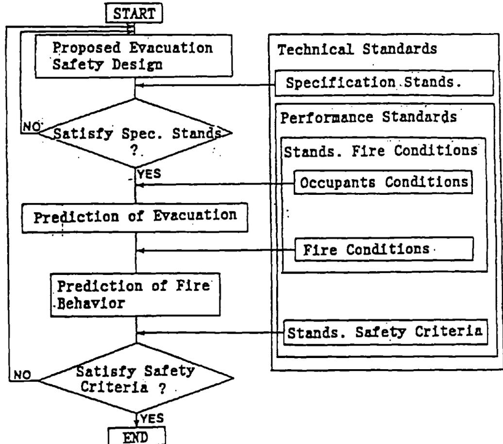
Figure 2. The Procedure of The Evacuation Safety Design
