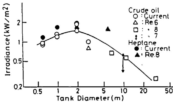
Figure 4 Relationship between radiative output and tank diameter
