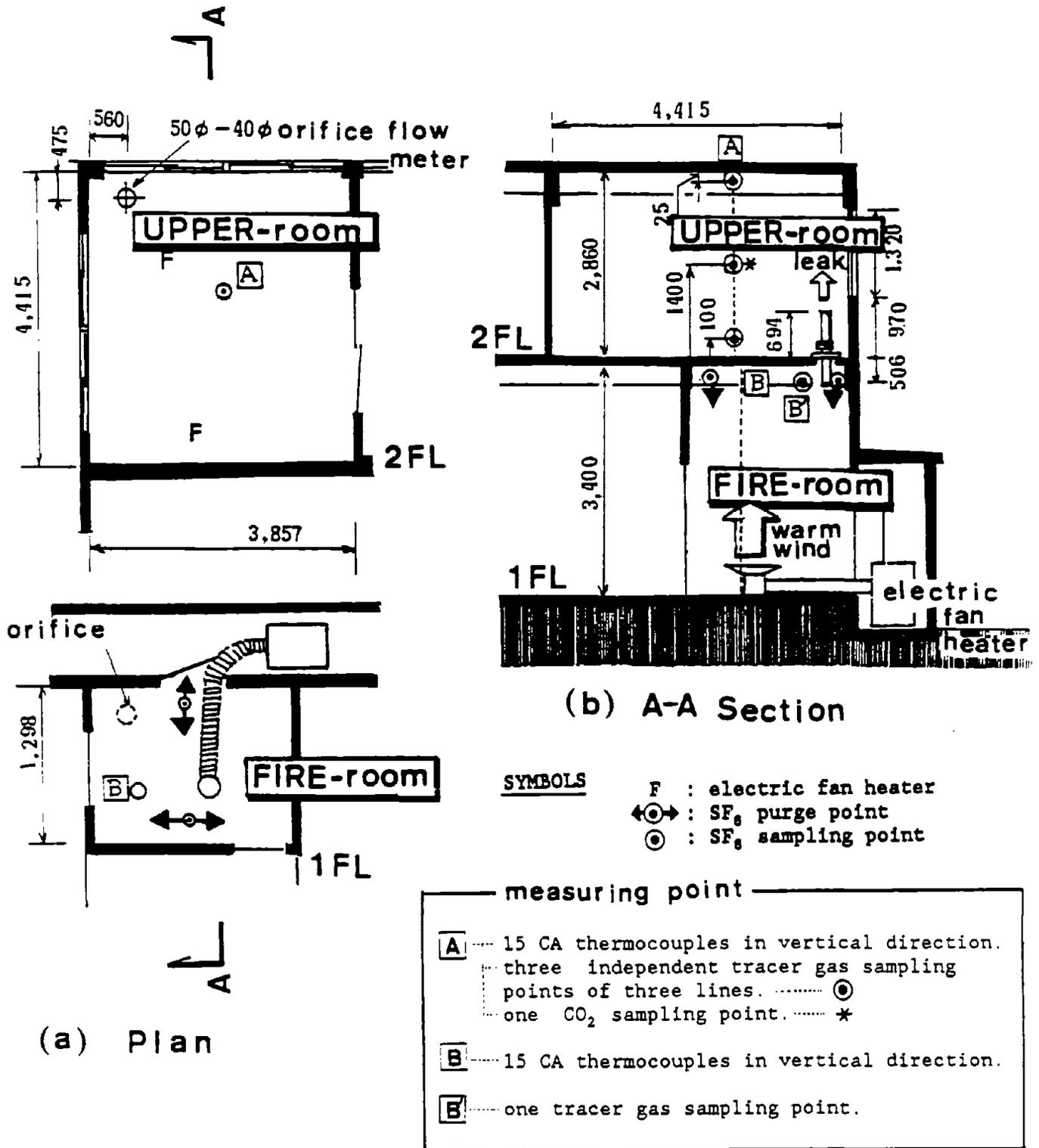
Fig.2. Instalation of full scale test ( series I ) ; A room on the 1st floor and another room directly above are supposed to be FIRE room and UPPER room respectively. Tracer gas is used instead of fire smoke to estimate leakage from FIRE-room to UPPER-room, while the leakage is measured by an orifice flow meter installed at a slab. pressure difference is produced by natural ventilation due to buoyant effect.
