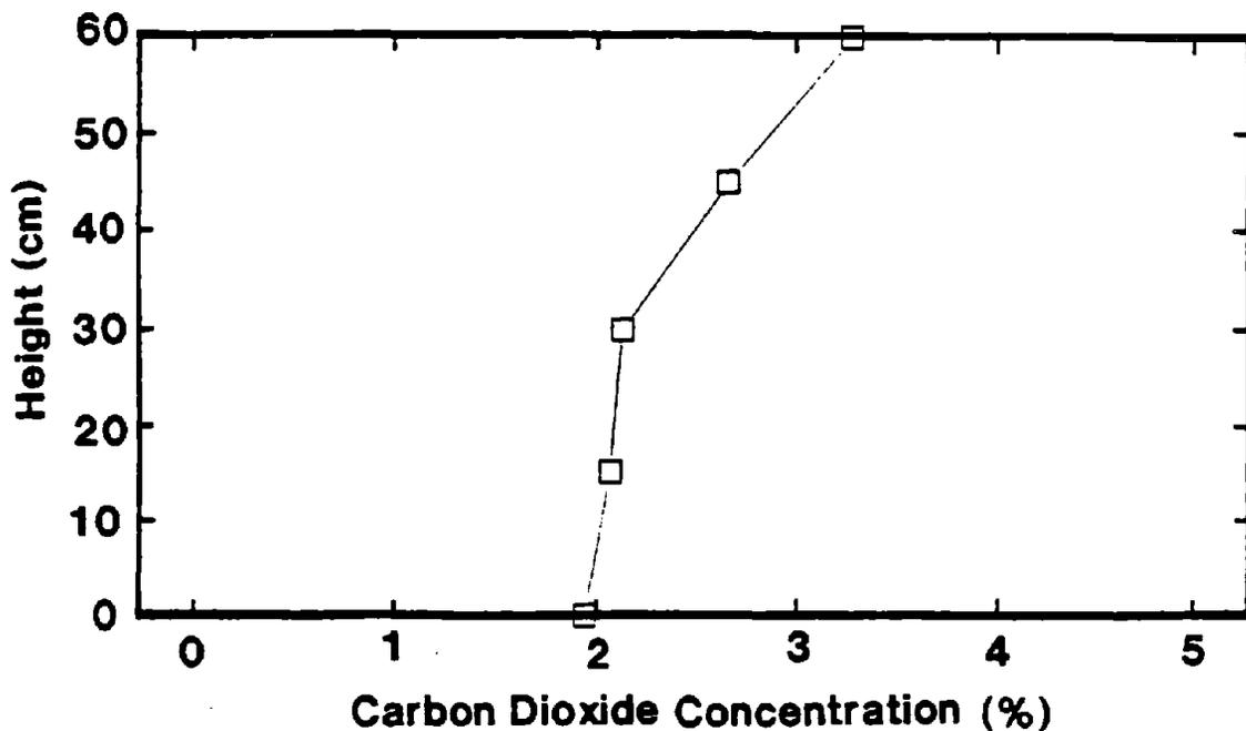
Figure 7 Vertical distribution of CO<sub>2</sub> gas concentration in the ghosting period. Data from Test 46.
