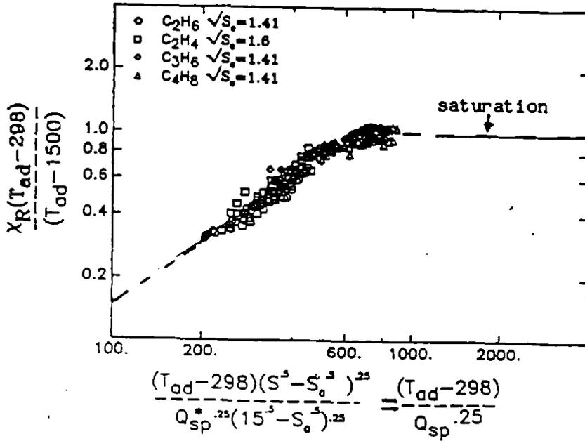
Fig. 3: Radiant fraction for varying adiabatic temperature and all S (the chemical system is Fuel - N<sub>2</sub>/O<sub>2</sub> - N<sub>2</sub>). S<sub>0</sub> is a characteristic cut-off stoichiometric ratio.
