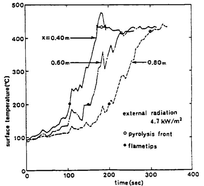
Figure 8 Time History of Surface Temperature ( $q_e^- = 4.7\text{kW/m}^2$ )
