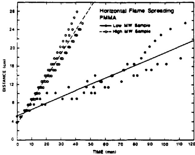
Fig. 5. Plot of flame front position with time for the PMMA samples.
