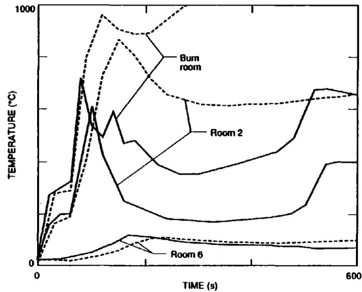
Figure 8. Average ceiling layer temperatures calculated using FAST 18 model of Sharon 2 test
