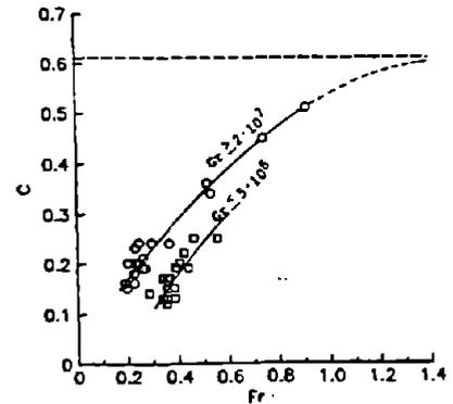
Figure 6 Discharge coefficients for ceiling apertures.
