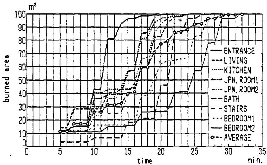
Fig. 7 Burned area-time curve by fire ignition room
