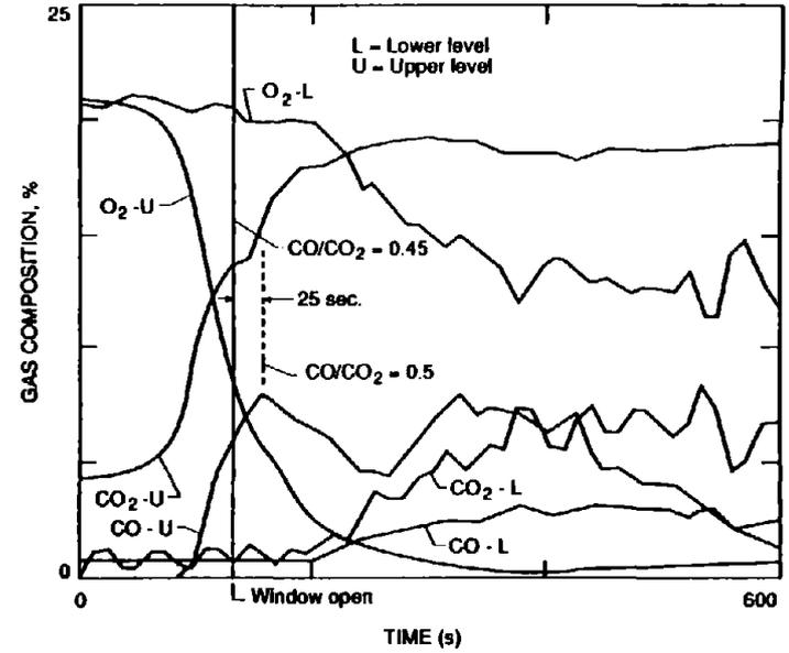
Figure 5. Gas composition of layer flows near burn room doorway Sharon 2 fire simulation
