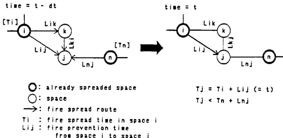
Fig.5 How to determine the fire spread time
