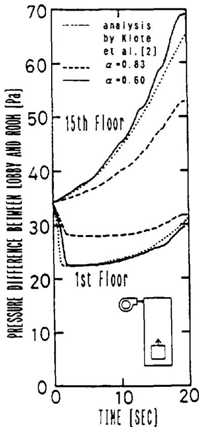
Figure-3. Comparison between the analytical results by Kote and Tamura and the calculation by the computing method when a cage ascends in a pressurized elevator shaft
