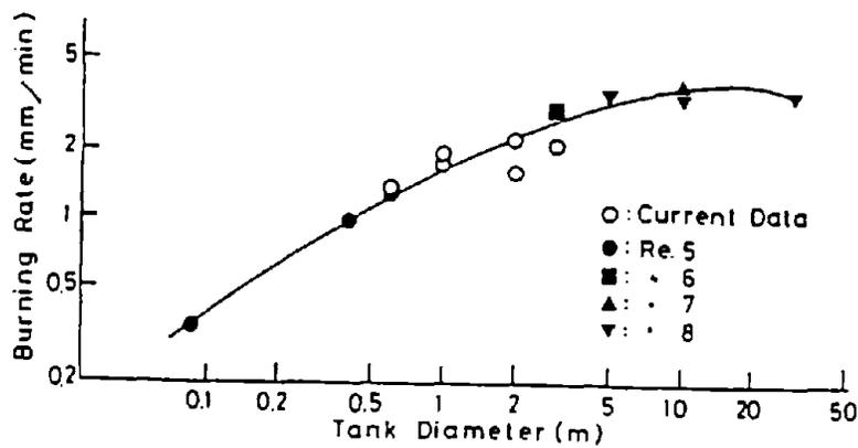
Figure 3 Relationship between burning rate and tank diameter
