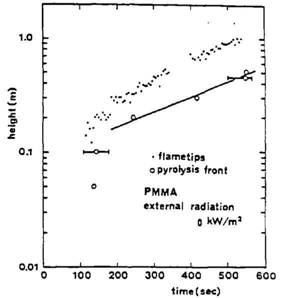
Figure 10 Location of Flametips and Pyrolysis Front
