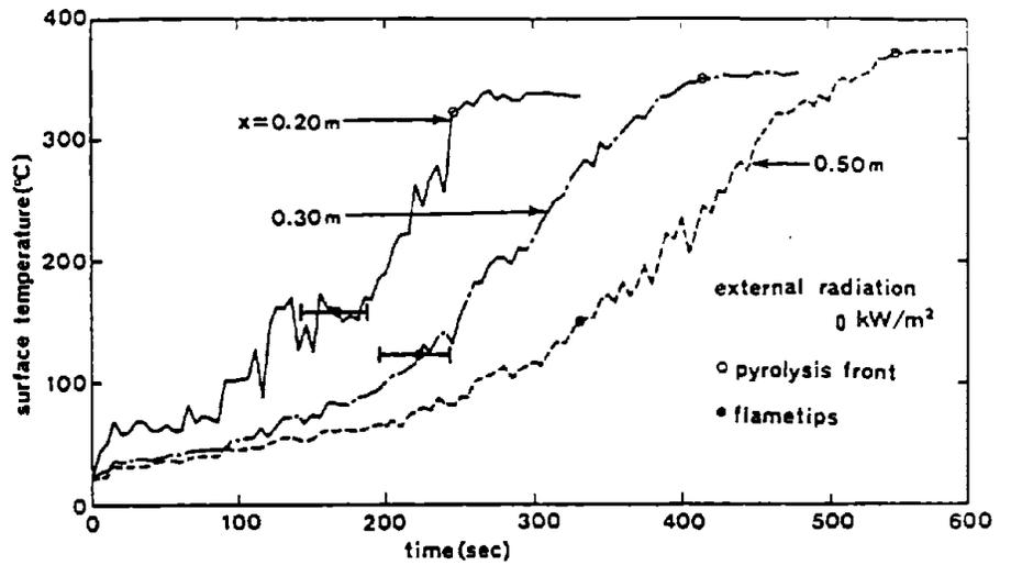
Figure 6 Time History of Surface Temperature ( $q_e^- = 0.0\text{kW/m}^2$ )
