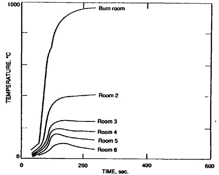
Figure 9. Average ceiling layer temperatures calculated using Harvard 6.3 model of Sharon 2 test
