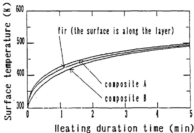
Fig. 2 Surface temperature histories of composites A and B, and fir.
