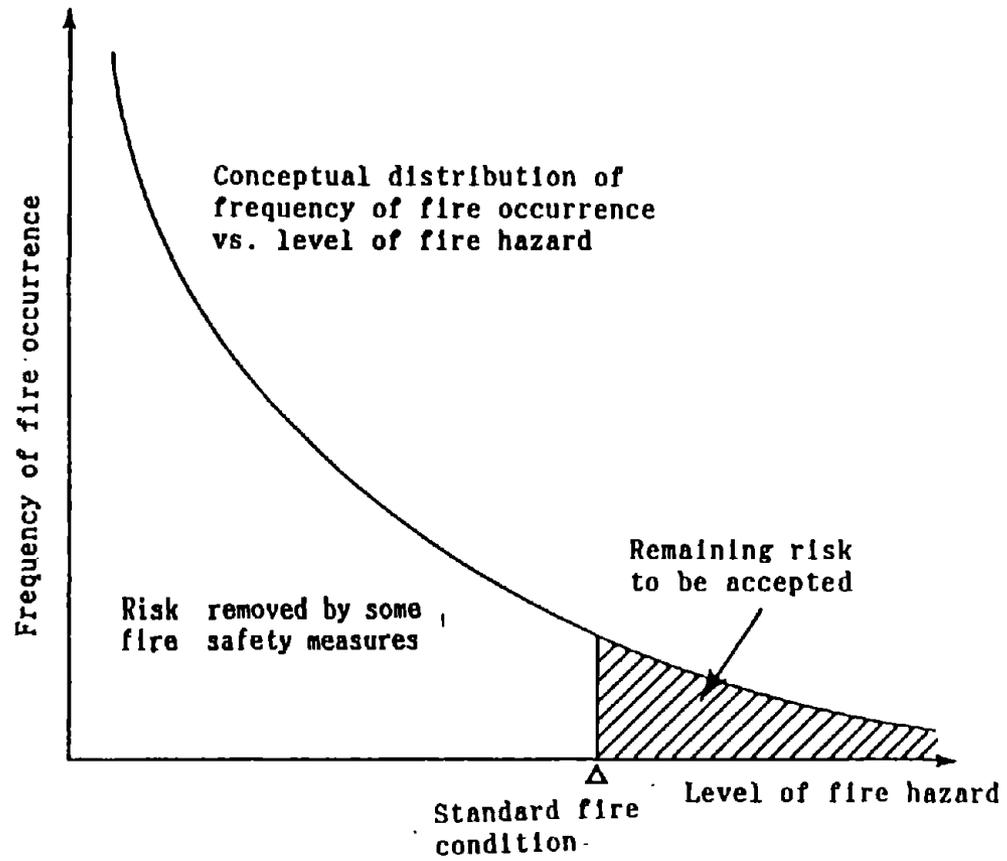
Figure 4. Meaning of standard fire condition
