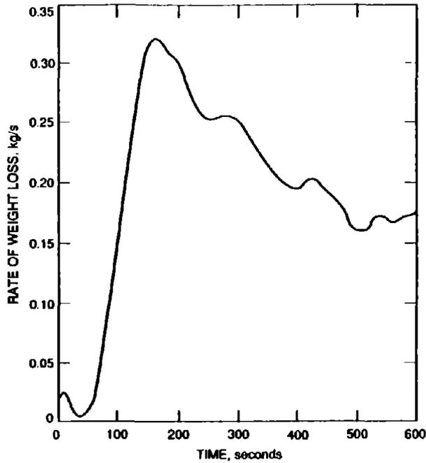
FIGURE 3. Rate of fuel weight loss Sharon 2 Fire Simulation
