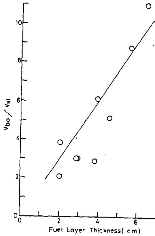
Figure 9 Relationship between  $V_{bo}/V_{st}$  and fuel thickness
