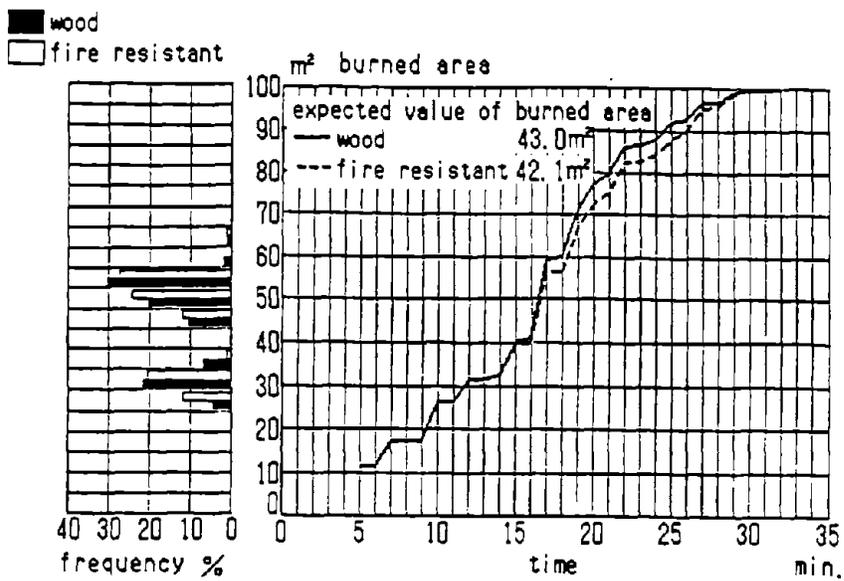
Fig. 6 Burned area-time curve and frequency of expected burned area
