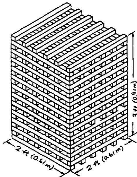
Figure 2. Crib configuration
