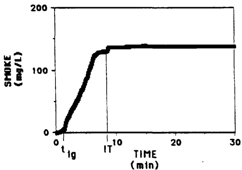
Figure 2. Typical Smoke Concentration - Time Curve
