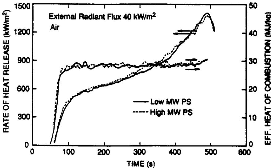
Fig. 9. Comparison of heat release rate and effective heat of combustion between the two  $\text{PS}_2$  samples at  $40 \text{ kW/m}^2$ .
