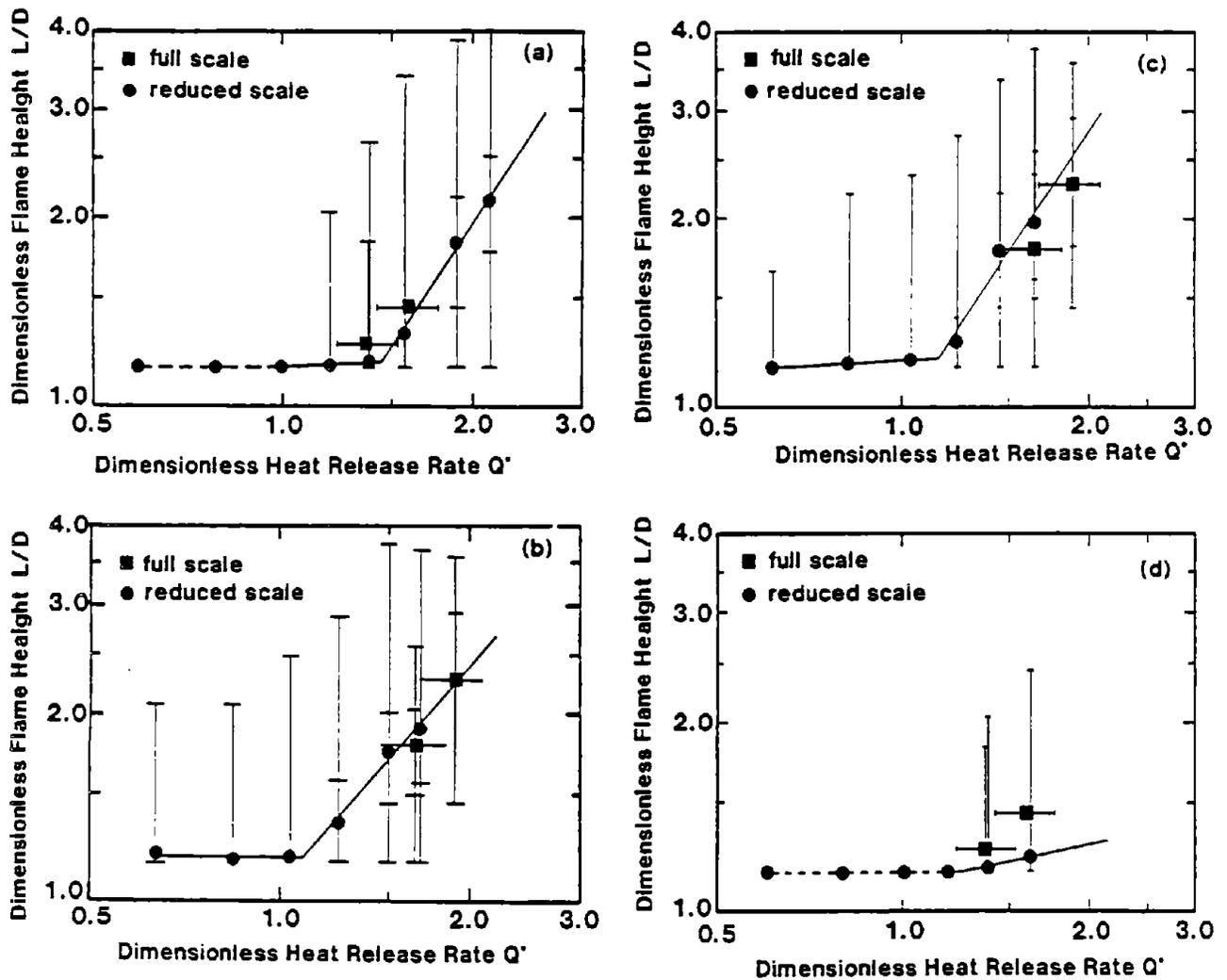
Figure 5 Correlation of the flame geometry ( $L/D$ ) versus  $Q^*$ , (a) no wind was given to the reduced model and fire source located at the end corner, (b) no wind was given to the reduced model and fire source located at the front of the opening, (c) wind was given and fire source located at the end corner, and (d) wind was given to the reduced model and fire source set at the front of the opening.
