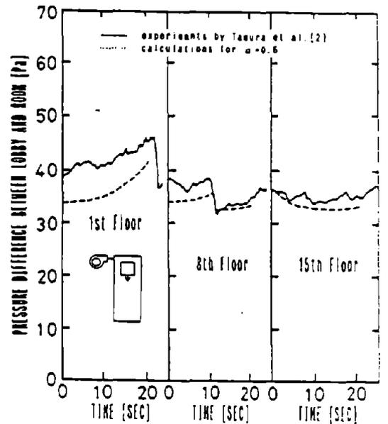
Figure-5. Comparison between the experiments by Kote and Tamura and the calculation by the computing method when a cage descends in a pressurized elevator shaft
