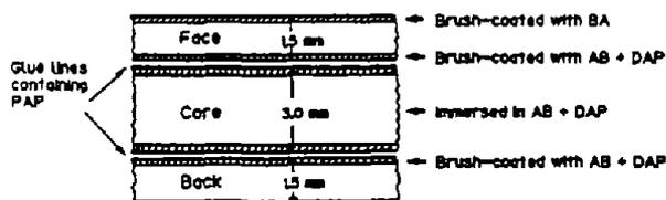
Fig. 1. Plywood sample.
