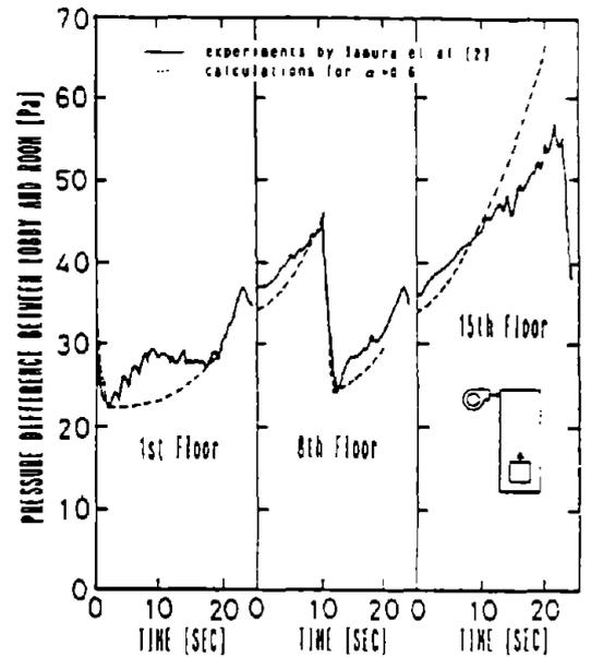
Figure-4. Comparison between the experiments by Kote and Tamura and the calculation by the computing method when a cage ascends in a pressurized elevator shaft
