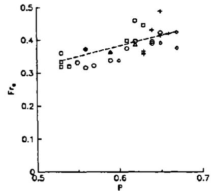
Figure 4 Critical Froude number for wall apertures;  $\circ$  floor-to-ceiling apertures;  $+$  high apertures;  $\Delta$  low apertures;  $\square$  central apertures;  $\ominus$  central circular aperture;  $\oplus$  doorway, larger-scale.
