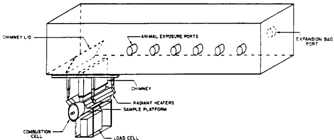
Figure 1. Schematic Drawing of Radiant Combustion/Exposure Apparatus
