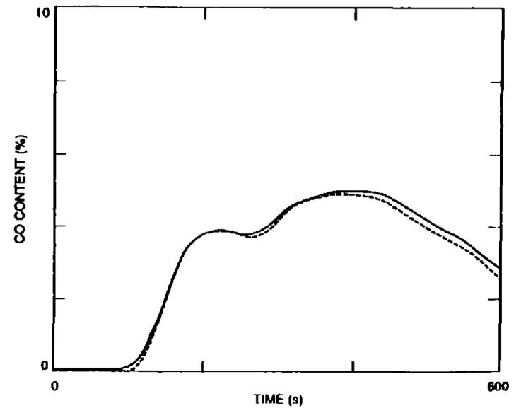
Figure 10. Comparison of CO concentration in ceiling layers of rooms 6 & 7. Measured data from Sharon 2 test
