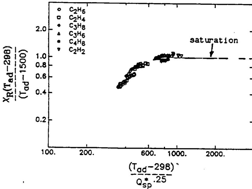
Fig. 2: Radiant fraction for varying adiabatic temperature and stoichiometric ratio  $S > 12$  (the chemical system is Fuel - N<sub>2</sub>/O<sub>2</sub> - N<sub>2</sub>)
