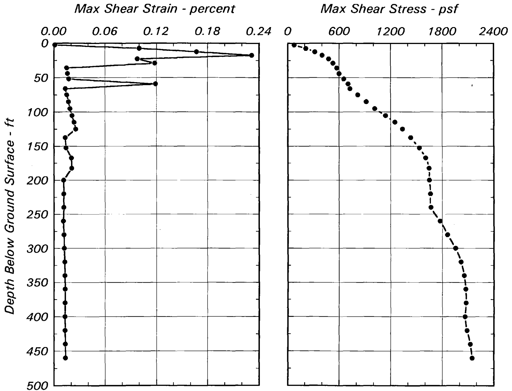
Fig. 4-5 Maximum Shear Strains and Stresses at SFO Calculated Using Best Estimate Shear Wave Velocities and Stronger Component of SP Record as Input Motion
