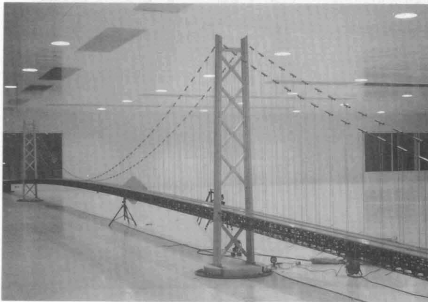
Photo 4 Full model test of the Akashi-Kaikyo Bridge
