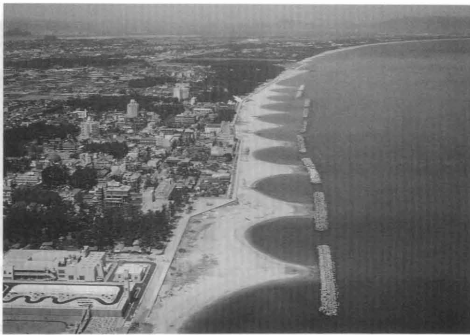
Photo 3 Detached Breakwaters and "Tombolo" at Kaike Beach
