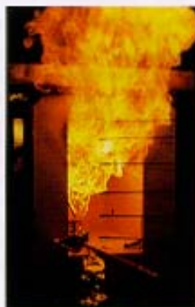
Scale model experiments to measure generation of carbon monoxide
