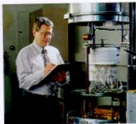
Robert Zarr checks the thermal conductivity apparatus
