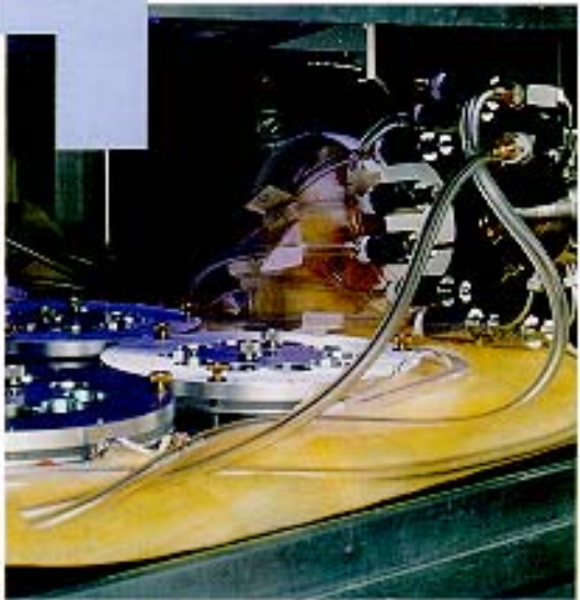
Apparatus for measuring photodegradation effects on polymeric material
