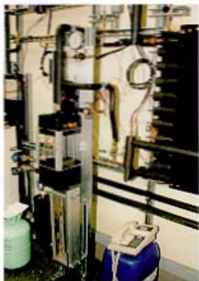
Distillation column, capable of changing refrigerant mixture composition in heat pumps
