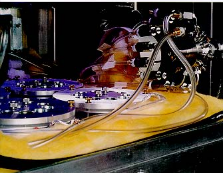
Apparatus for measuring photodegradation effects on polymeric material
