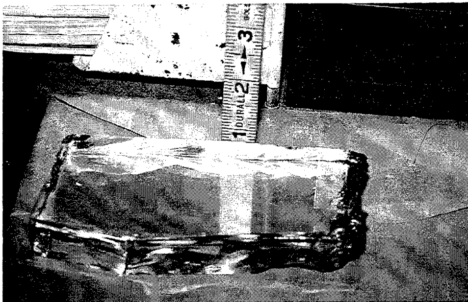
Fig. 10.3 Fragment of control tower window glass that is 3/4" (2 cm) thick.
