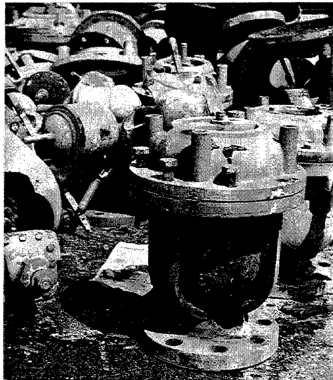
Fig. 4.18 Broken air and vacuum valves.
