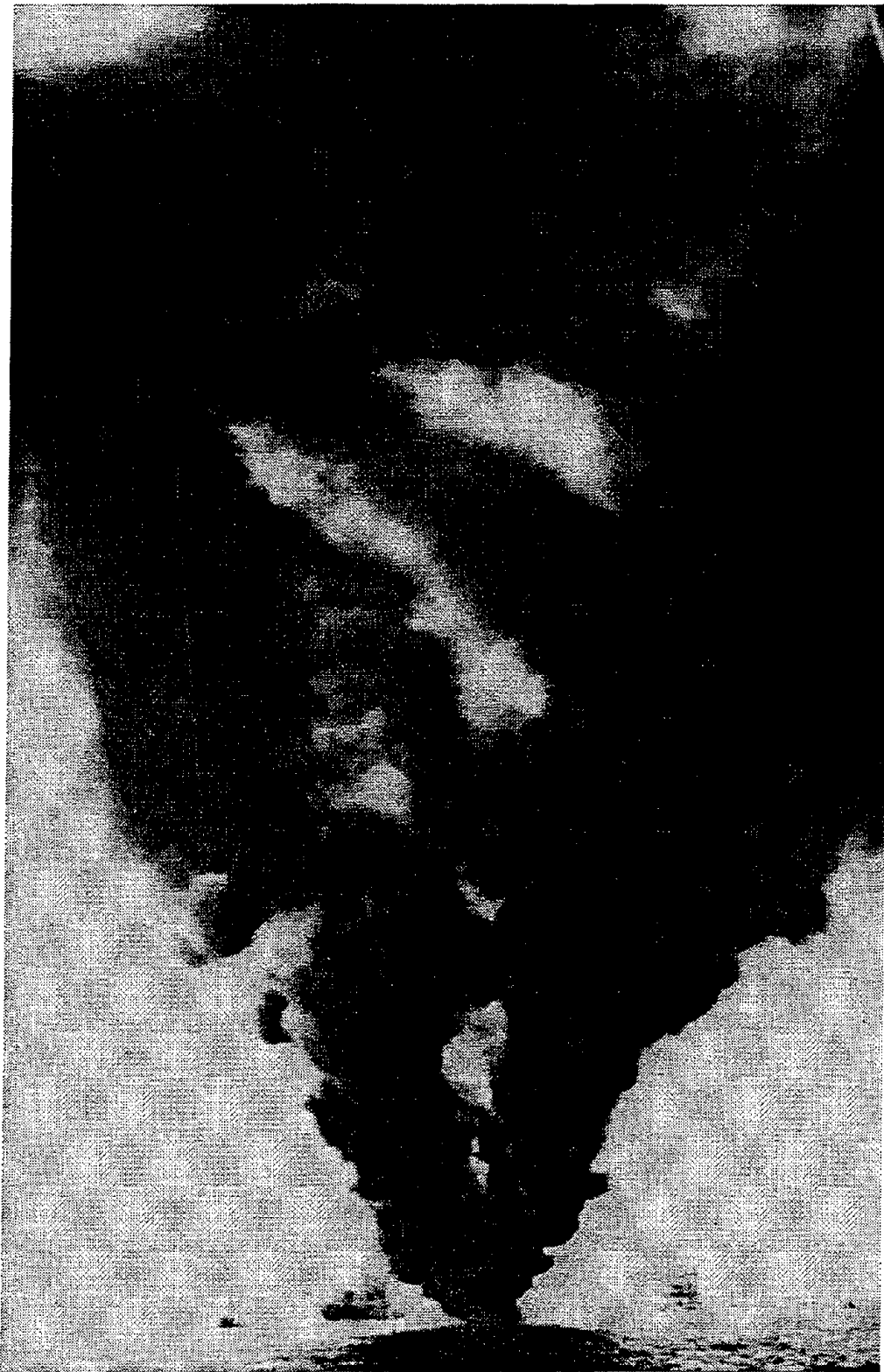
Figure 3: Photograph taken from about 200 m downwind of the Newfoundland Offshore Burn Experiment (NOBE) showing the two large counter-rotating vortices which characterize the structure of the rising smoke plume.
