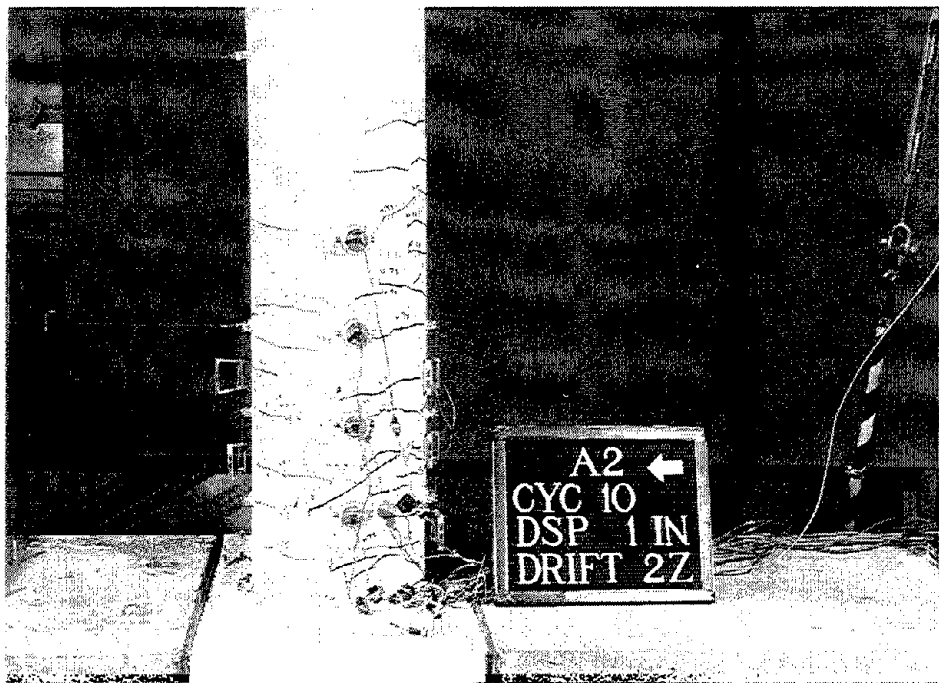
FIGURE 2-21 Clip Gage Mounted on Column for Curvature Measurement
