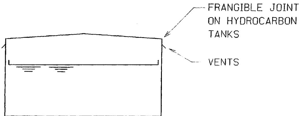
CONE ROOF WITH INTERNAL PAN
