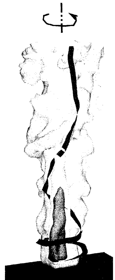
Simulations of a fire plume showing three major zones: the continuous flame (red), the intermittent region (yellow), and the plume region (gray).
