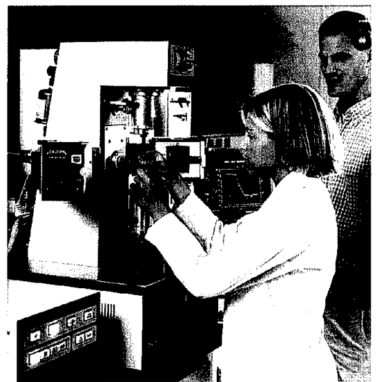
Dr. Mark Van Landingham, materials research engineer, and Ms. Amanda Grasso, student, prepare a specimen for dynamic mechanical analysis. DMA characterization of tape adhesives was used in the consortium study.
