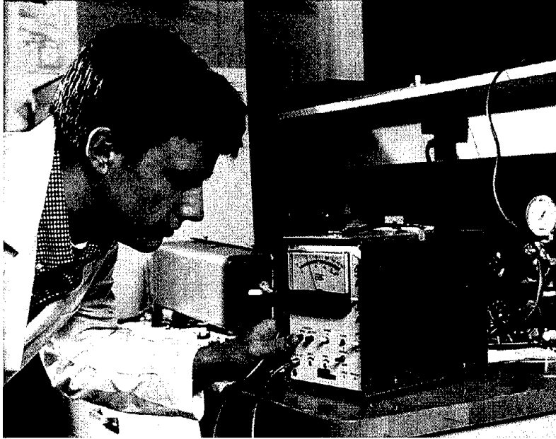
Mr. Kevin Denton, coop student at the University of Maryland, prepares a carbon dioxide monitor for field measurements of indoor air quality in an office building as part of meeting the C&B program goal of achieving a 50 percent reduction in occupant related illnesses and injuries.
