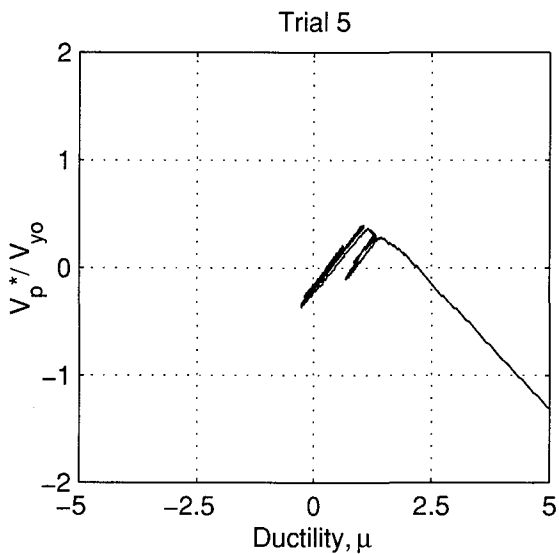
FIGURE 4-94 Specimen 14 – Normalized Base Shear vs. Ductility
