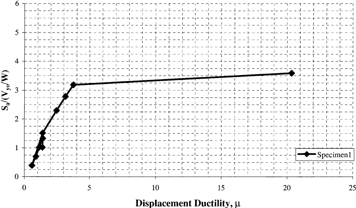
(b) S_a/(V_{y0}/W) vs \mu ( 0.1 < \theta \leq 0.3 )
