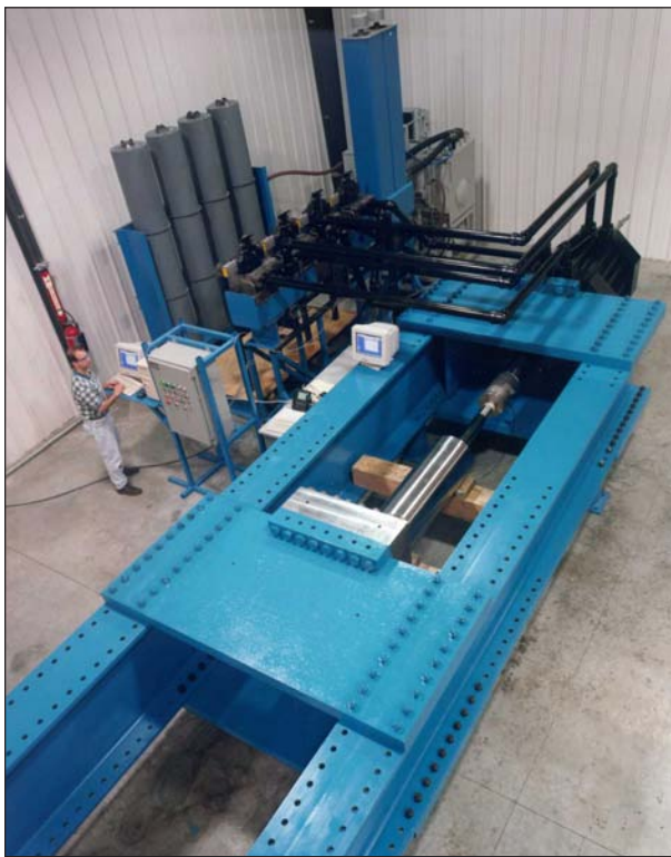
■ Figure 10. 1.5 million lb. load frame at the Taylor Devices Testing Facility
