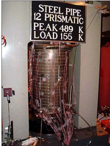
■ Figure 4. Prismatic pipe specimen in load frame
