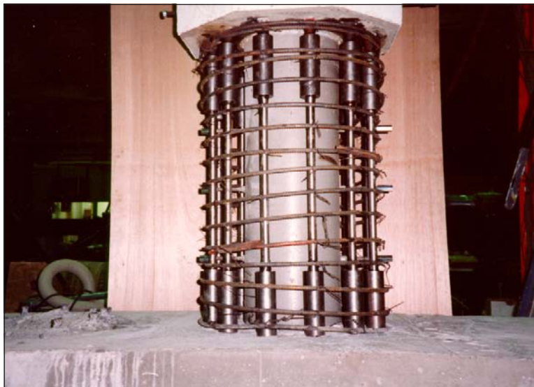
Undamaged specimen (prior to testing)
