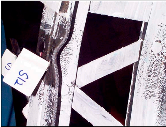
Figure 21. Buckling for Ay8-60
