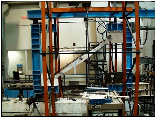
Figure 5. Test set-up for specimen Ay16-60
