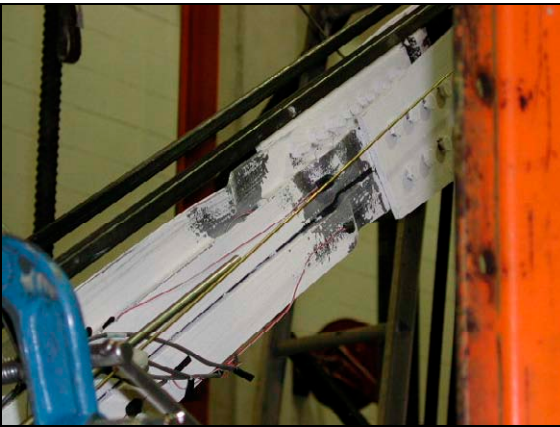
Figure 23. Buckling for Ay16-60
