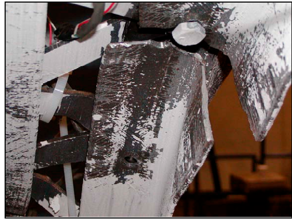
Figure 24. Fracture of Ay16-120
