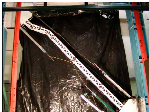
Figure 20. Global buckling for Bx8-120
