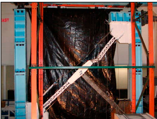
Figure 19. Global buckling for Bx8-60
