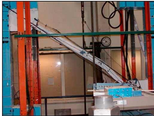
Figure 18. Global buckling for Ay16-120
