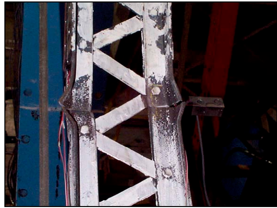
Figure 22. Fracture of Ay8-120
