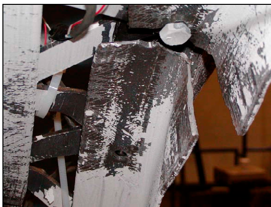
Figure 25. Buckling of Bx8-60
