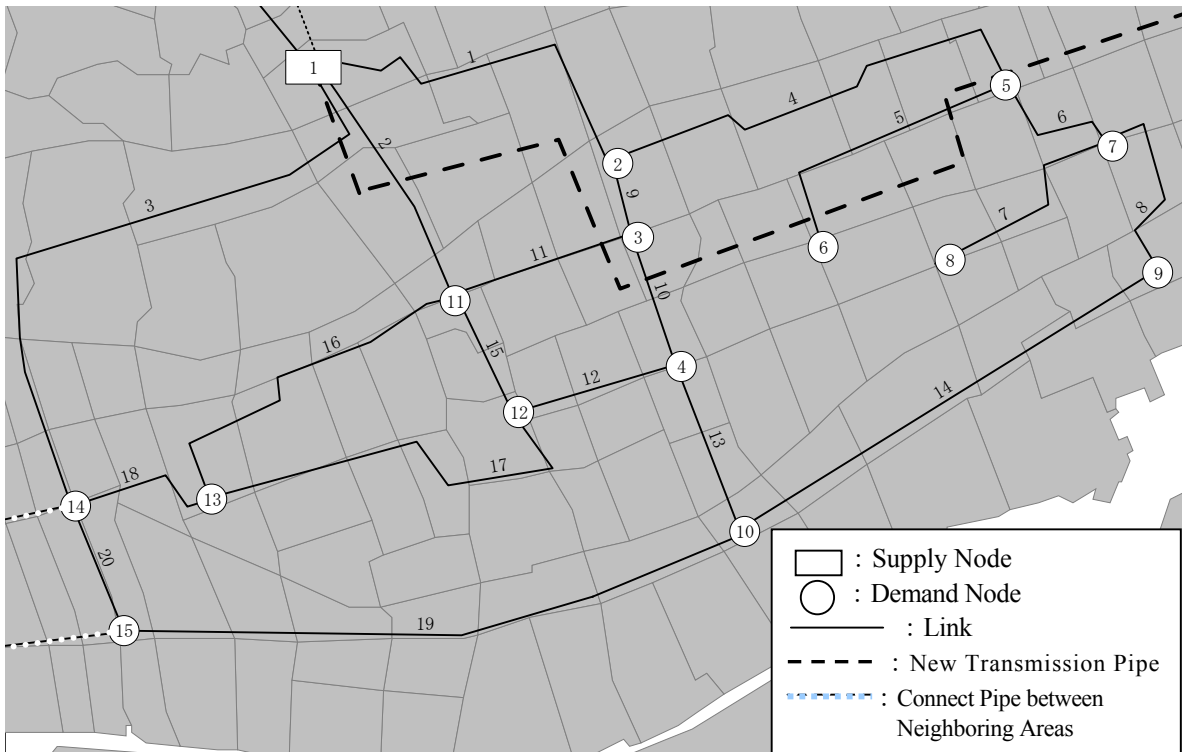
Figure 3. Water supply network of distribution area A.
