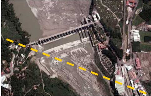
Figure 6: Failure of Shihkang dam due to faulting
