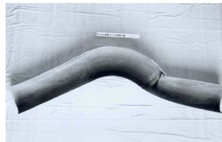
(b) Opening mode bending (X52, Dn=400mm, D/t=51, R=1.5D, \phi=22.5^\circ )
