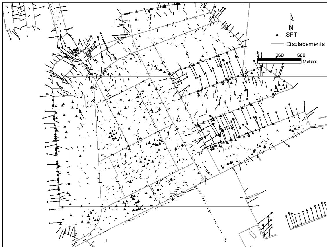
Figure 4. Displacement vector and borehole location in Port Island (data after Tanaka and Okimura, 2001)
