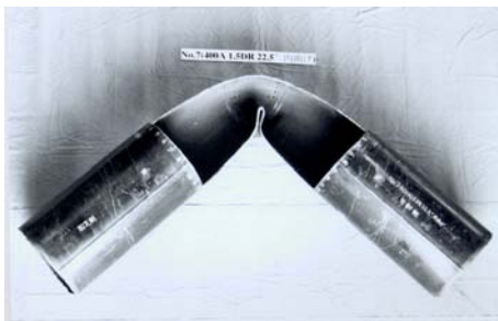
(a) Closing mode bending (X52, Dn=400mm, D/t=51, R=1.5D, \phi=90^\circ )
