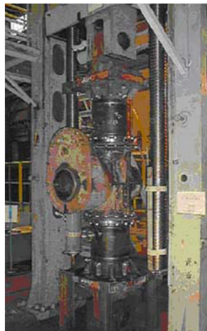
Photo 1. Tensile Strength Tests for Cast Iron Valves
