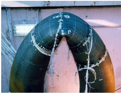
(a) Closing mode bending (X65, Dn=600mm, D/t=40, R=3D, \phi=90^\circ )
