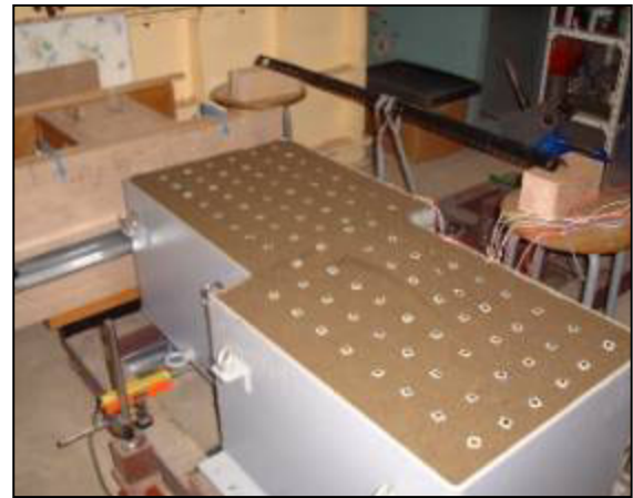
Photo.7 Shear deformation of the soil box with a buried pipeline
