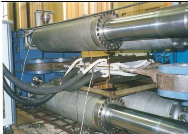
Figure 11. ExxonMobil Wide Plate Tests to Assess Strain Capacity of Girth Welds
