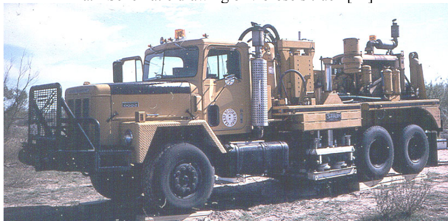
b. Vibroseis truck at field test site in Austin, Texas
