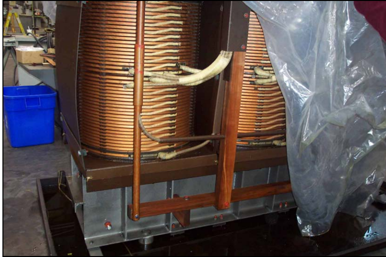
Figure 5. Internal components of a transformer
