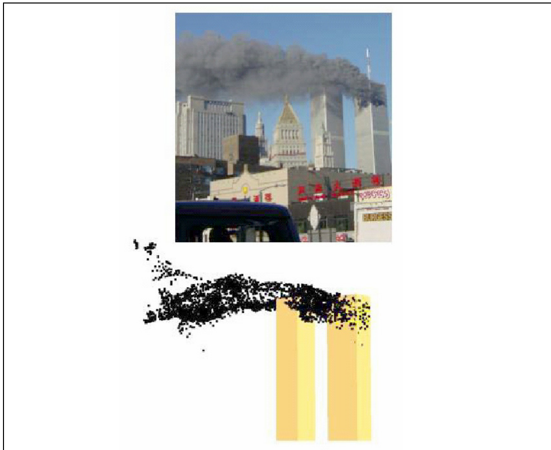
Figure 3-3. Comparing a photograph with the simulated plume for WTC1
