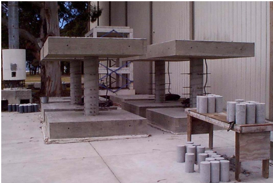
Figure 3-22. The four specimens after form removal.
