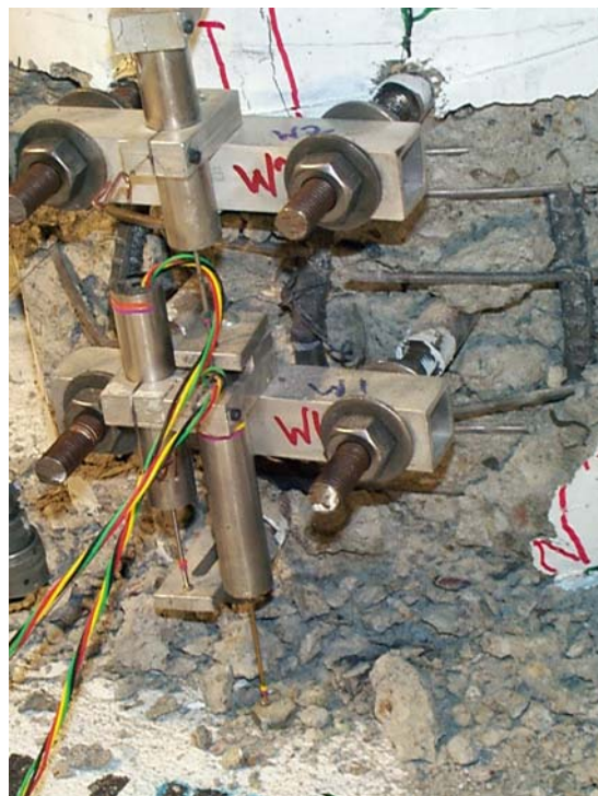
Figure C-36. Specimen A1 after Run 8. Another view of the west face with the fracture bar (#9).
