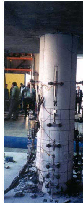
Figure C-70. Specimen B2 after Run 8 (north face).
