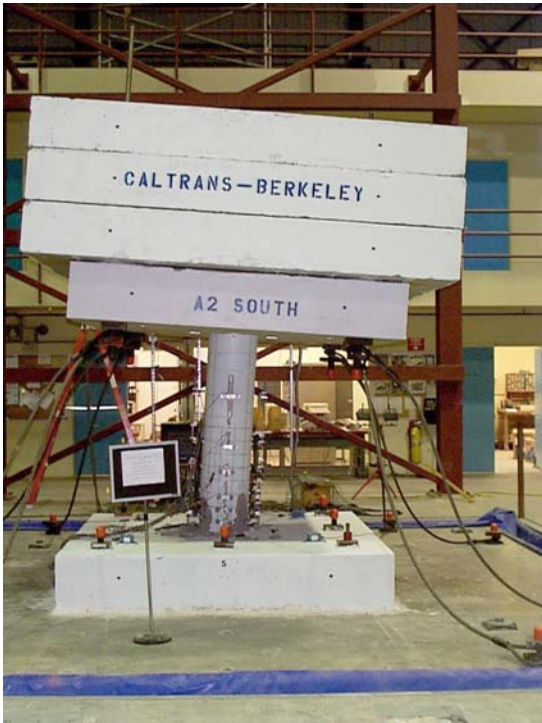
Figure C-53. Specimen A2 at the end of the last run (Run 10). The column had a residual displacement of about 6 inches (at the mass center).
