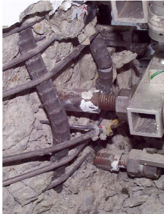
Figure C-34. West face of specimen A1 after Run 8. One fractured bar (#9), a buckled bar (#10), and a fractured spiral are shown.
