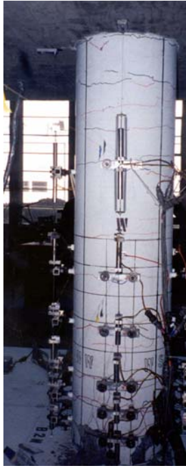
Figure C-67. Specimen B2 after Run 8 (west face).
