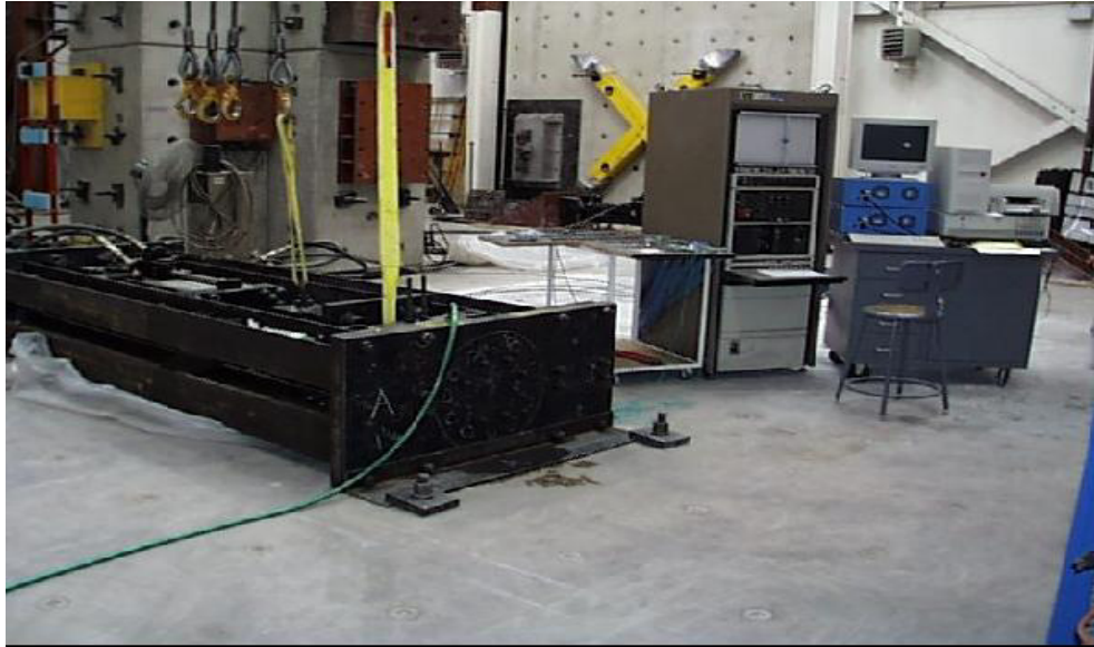
Figure 2-1 Load Frame and Actuator Configuration for Static Load Testing
