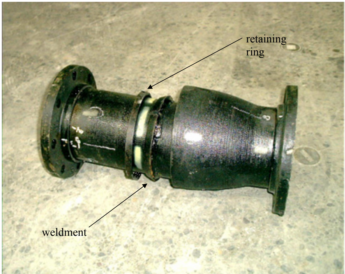
Figure 1-12 Ductile Iron Pipe with Retaining Ring
