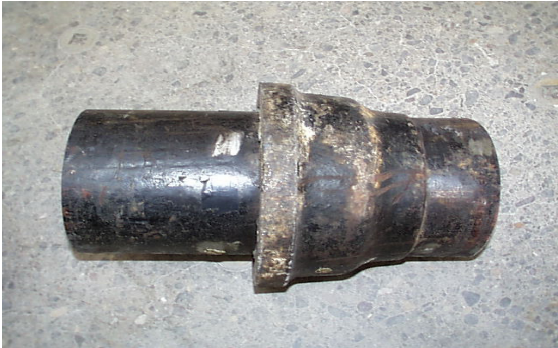
Figure 1-10 Cast Iron Pipe with Lead-Caulked Joint
