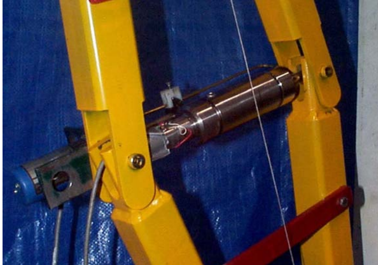
Figure 3-4 Close-up of Damper-to-Brace Connection Detail
