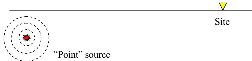
Figure 4-1 Fault-Site Model for Earthquakes in ENA
