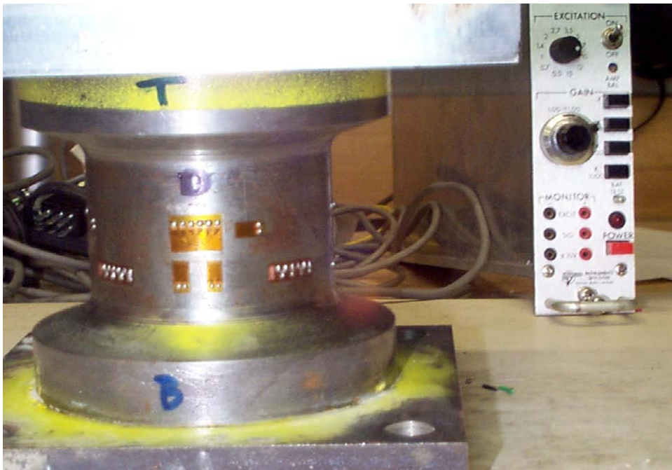
Figure F.7 View of Gauges and Terminals
