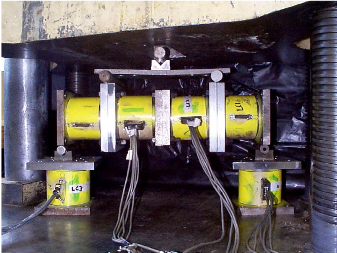
Figure F.9 Actual Load Cell Calibration Setup
