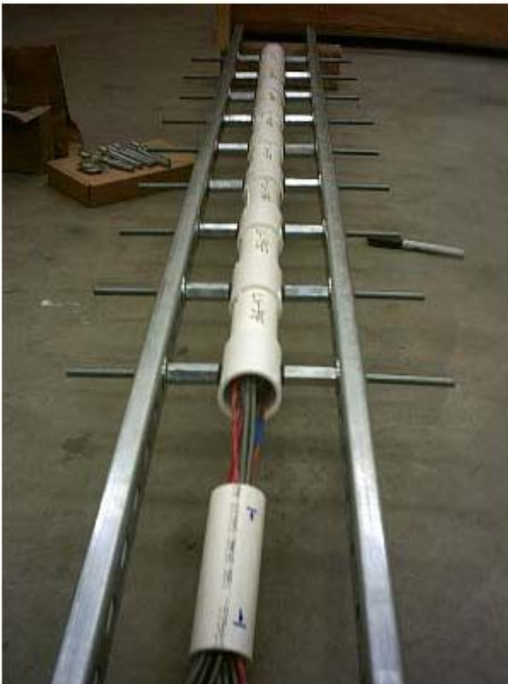
Figure 6. Axial LVDT assembly
