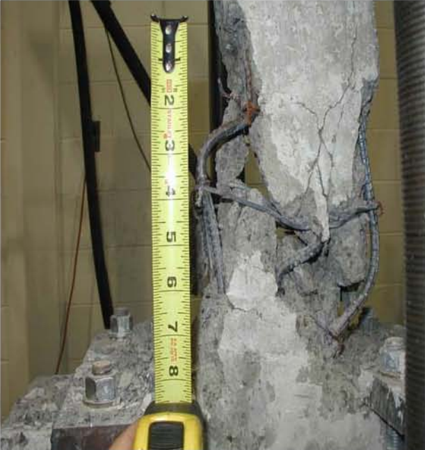
Figure 7.5: Progression of damage in specimen 2. a. Shear failure. b. Axial load failure.
