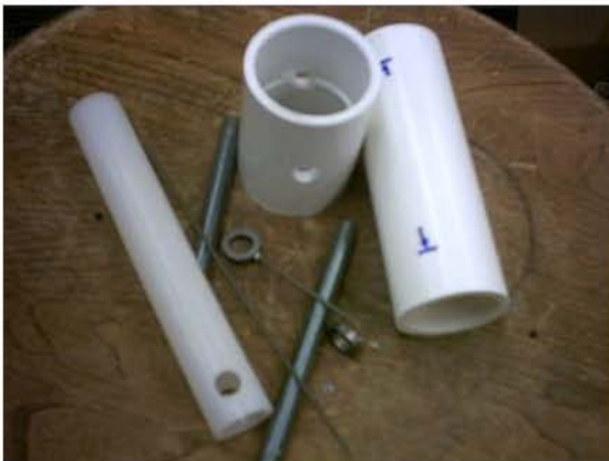
Figure 4. Pieces for the LVDT casing
