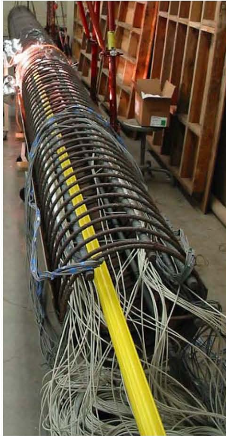
Figure 11. Column with wiring
