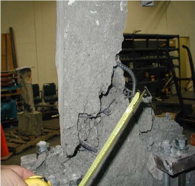
Figure 7.5: Progression of damage in specimen 2. a. Shear failure. b. Axial load failure.
