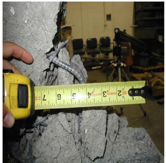
Figure 7.6: Specimen 2 damage at axial load failure.
