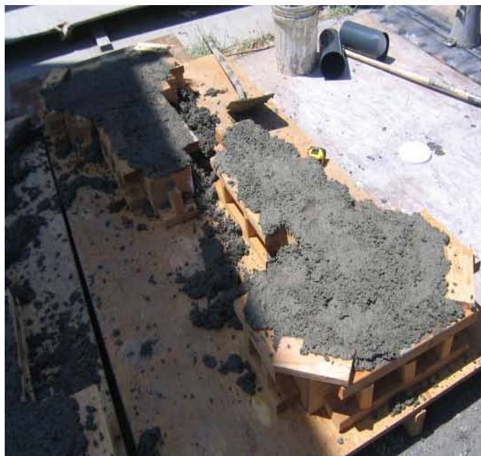
Figure 6.4: Casting of test specimens.
