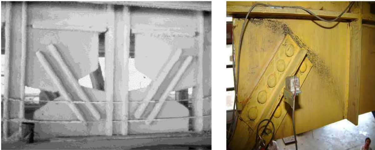
Figure 2: Oversized Gusset Plate Connections Used in SCBF
