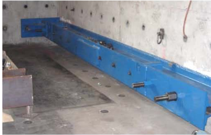
Figure 6: Channel Section Tensioned to Strong Wall
