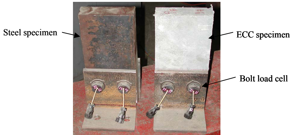
Figure 3-12. Steel and ECC specimens used to examine time dependent loss of bolt tension
