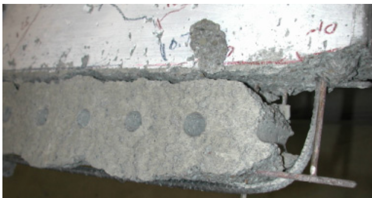
Figure 4-34. Connection region of Panel 5 after completion of testing
