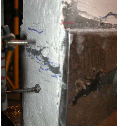
Figure 5-15. Cracking in connection region of Panel 1 during test
