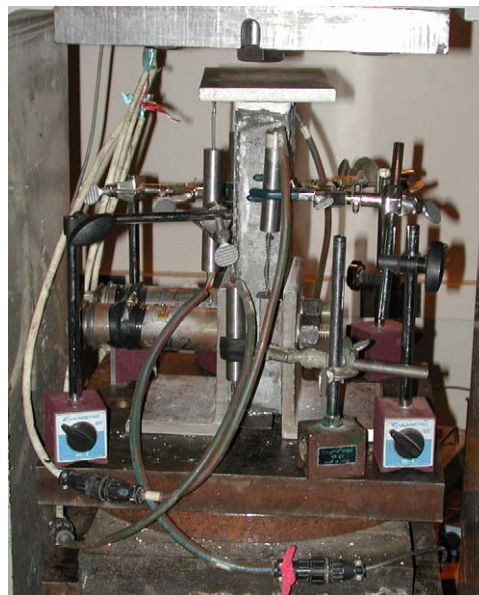
Figure 3-5. ECC connection specimen in test frame with LVDTs prior to testing
