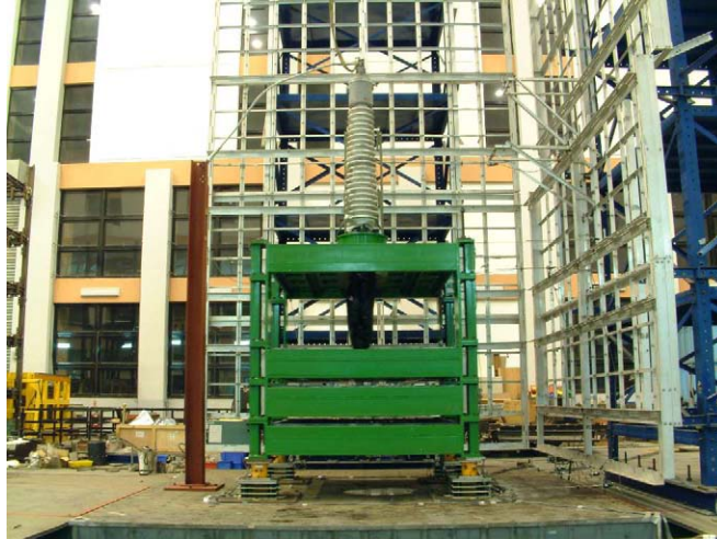
Figure A-1 Cable-Connected Base-Isolated Transformer Model
