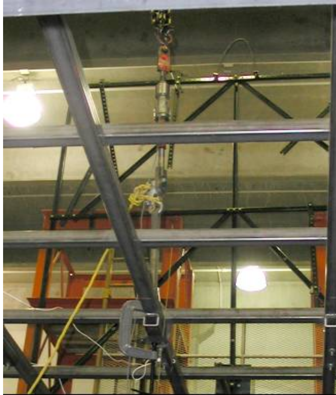
FIGURE 4-3 Configuration of the snap-back test in the vertical direction
