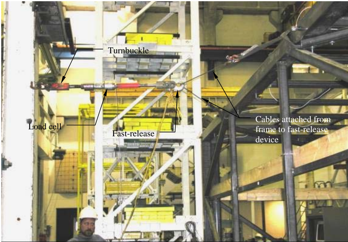
FIGURE 4-1 Configuration of the snap-back test in the horizontal direction
