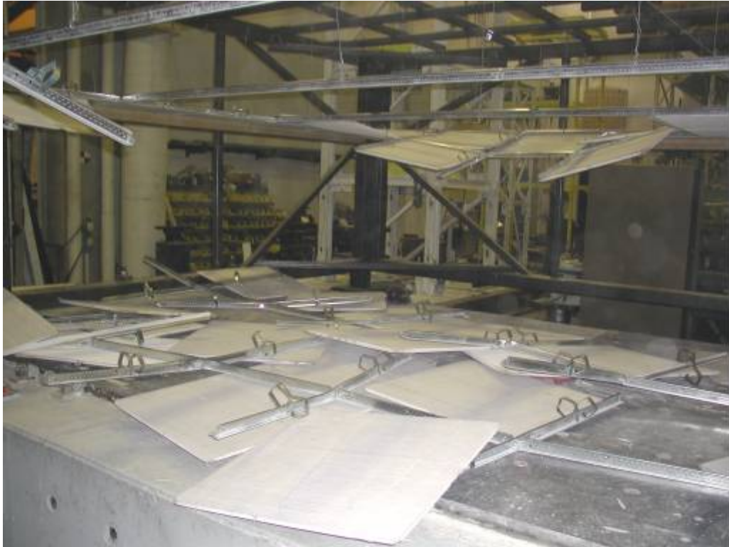
FIGURE 6-11 Failure of grid and tiles in configuration 5
