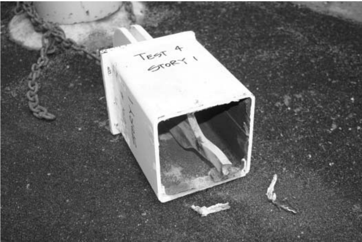
Figure 4.74. SSBRB After Fracture
