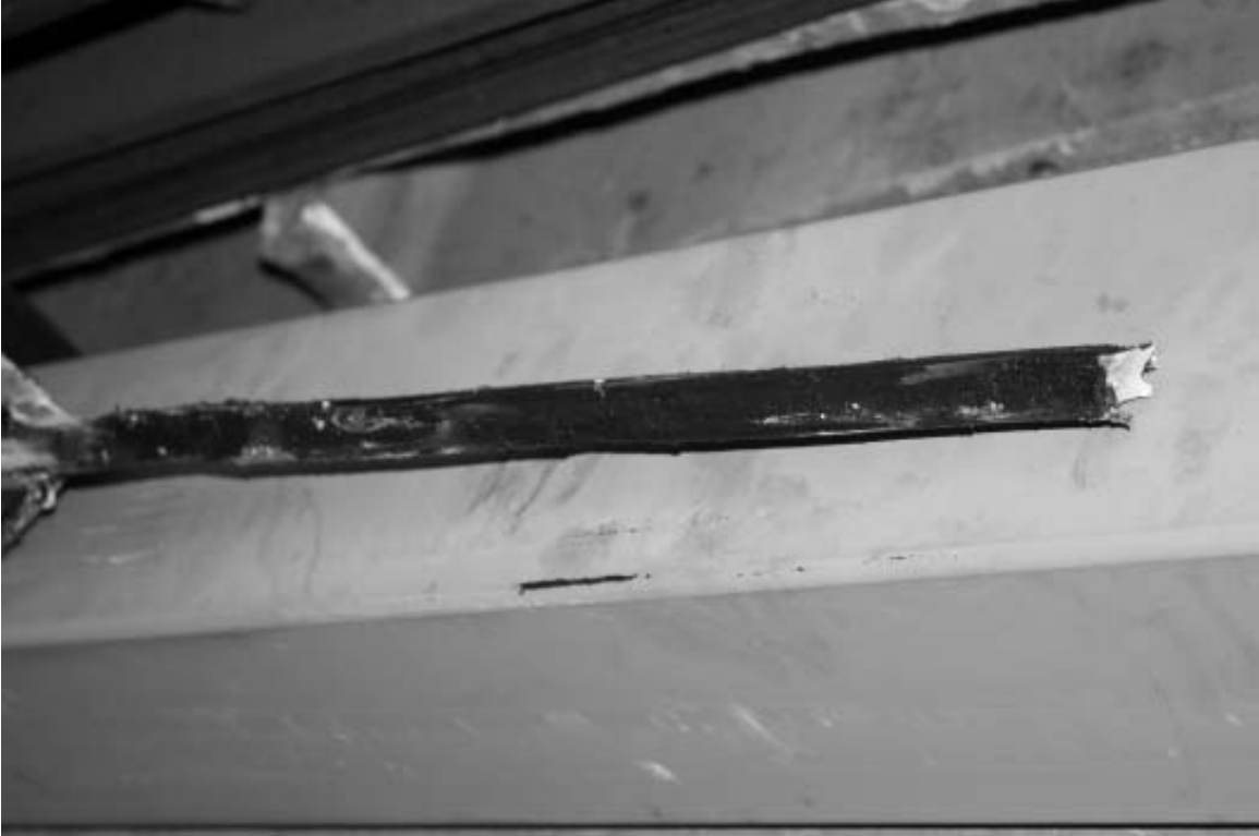
Figure 4.73. NSBRB After Fracture
