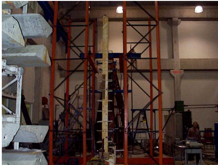
(c) Stabilizing Frame Setup
