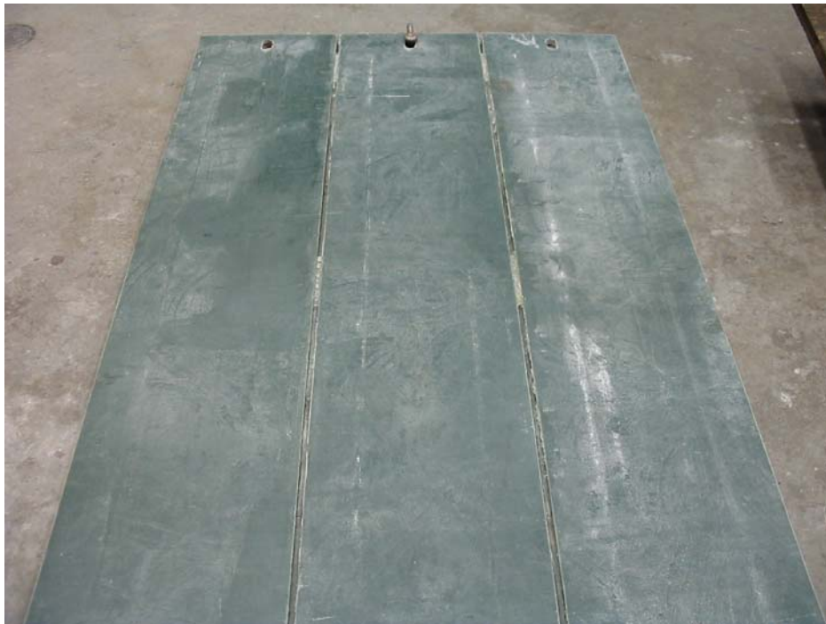
Figure 6-19 View of the Outer Damping Panel
