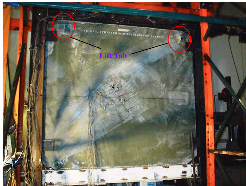
Figure 6-13 Fabrication of the PMC Sandwich Infill Panel
