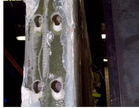
(b) bolting joint sliding of outershell
