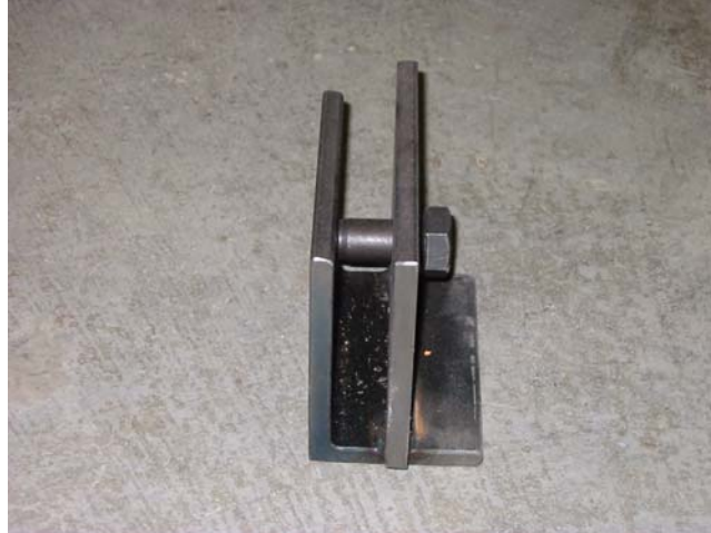
(a) Fabricating Beam-to-panel Connector
