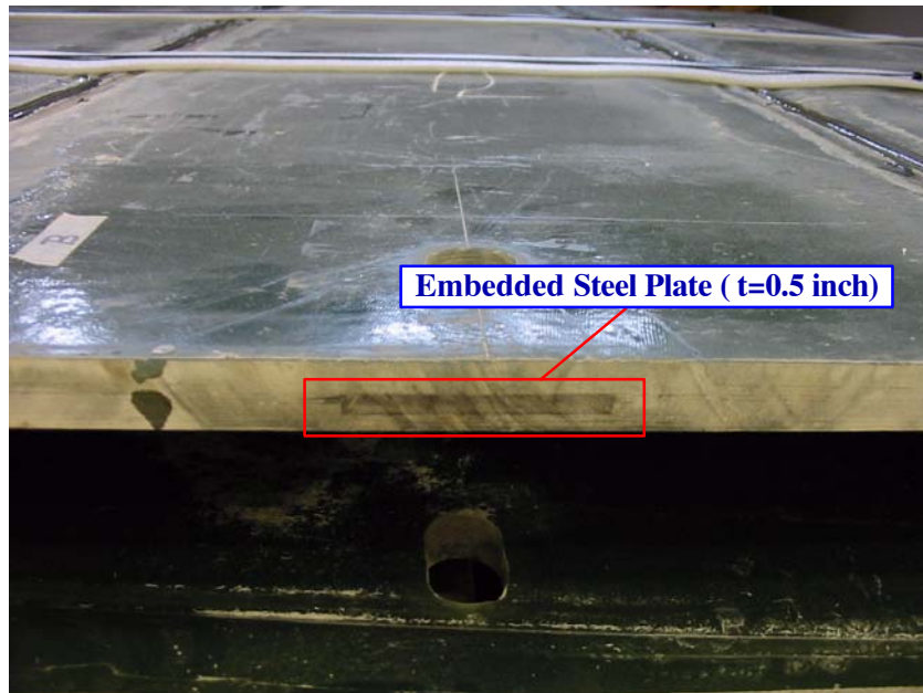
Figure 6-30 Sandwiched Steel Plate in the FRP Box Panel
