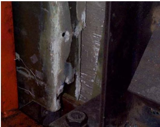
(c) outershell spalling off - bolting release
