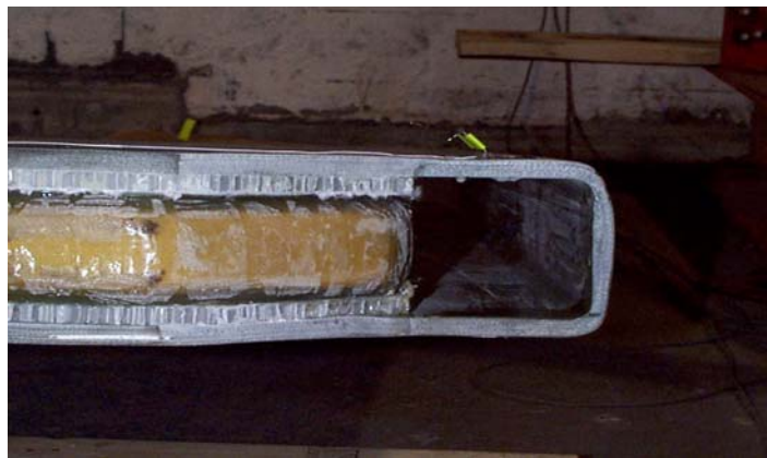
(b) Rounded Edge of the Multi-layer PMC Infill panel
