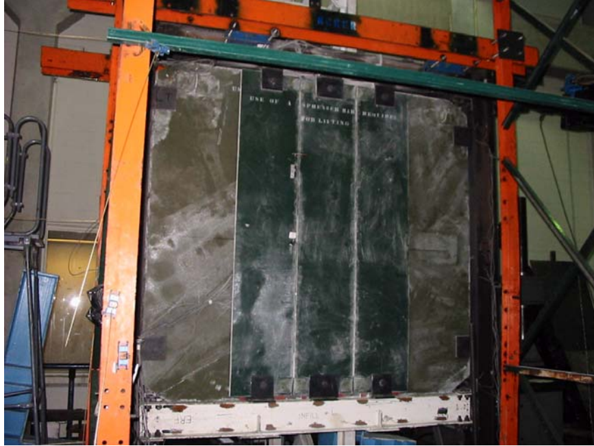
Figure 6-36 Multi-panel PMC Infill Panel Setup
