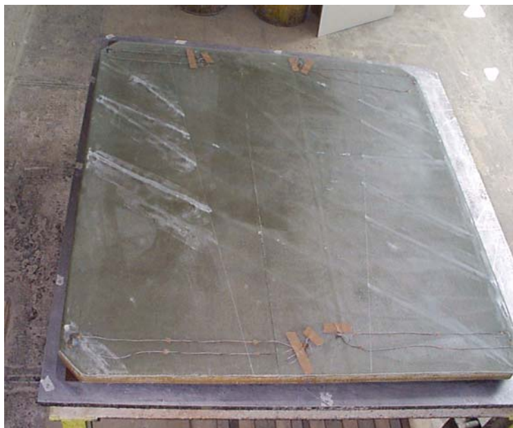
Figure 4-16 Inner PMC Sandwich Composite Panel
