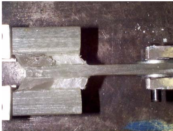
(c) Bonding Failure of Honeycomb
