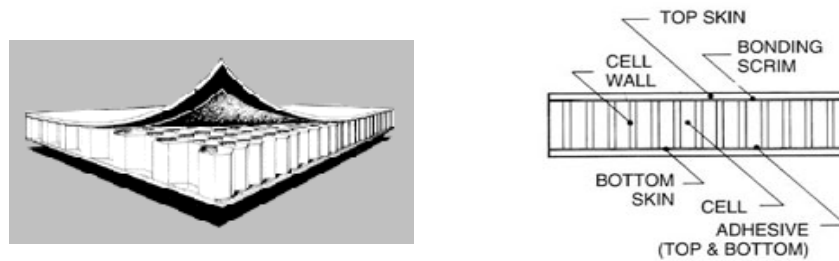
Figure 5-1 The Structure of the Honeycomb Material
