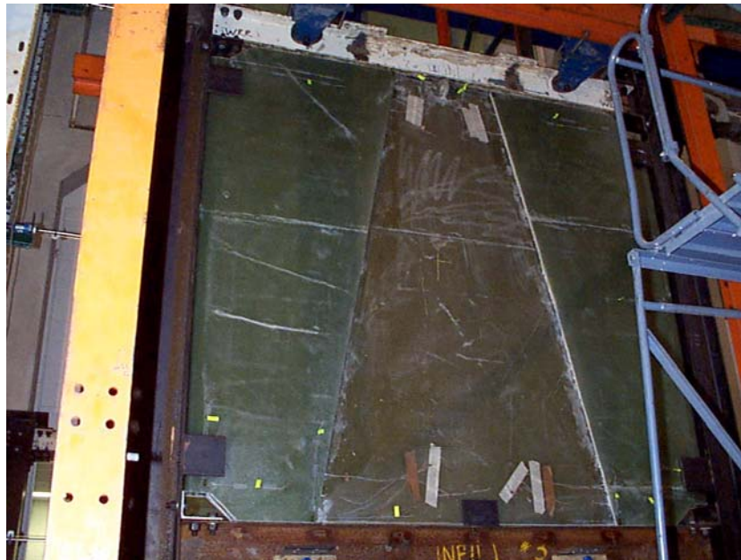
Figure 4-20 Multi-layer Infill Panel Setup
