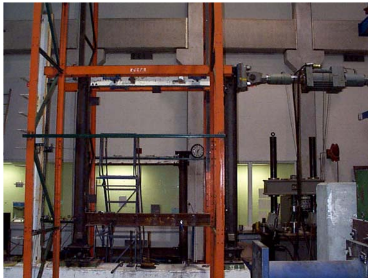
Figure 3-4 Steel Frame Setup
