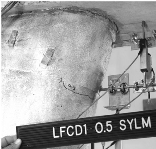
Fig. 4-3 LFCD1 at 0.5 times Sylmar (a) Joint Cracks (b) Flare Cracks
