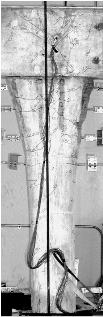
Fig. 5-16 LFCD2 Crack Pattern after Bucket Removal
