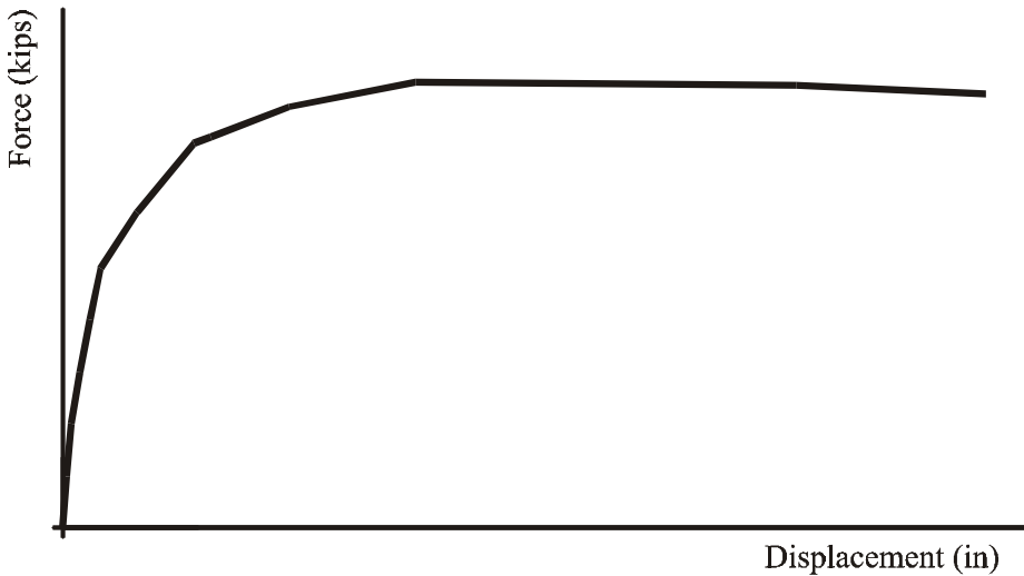
Fig. 4-12 Typical Load-Displacement Curve for PBD Bents
