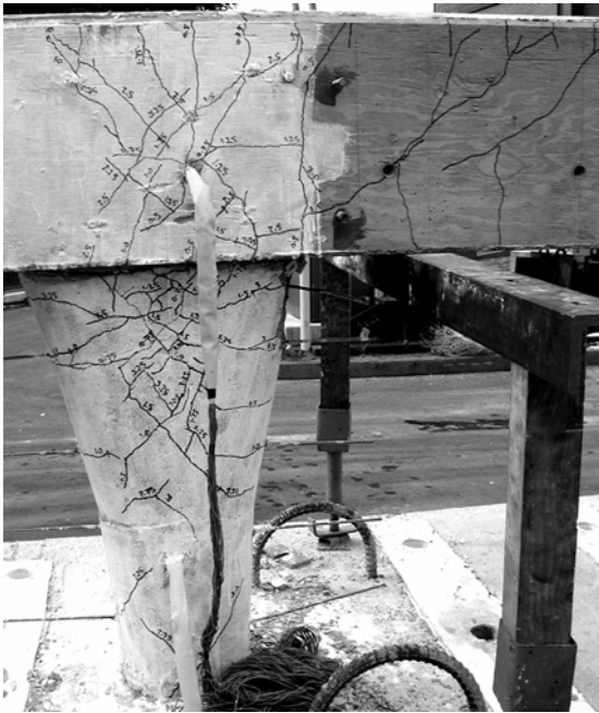
Fig. 4-116 After Bucket Removal Cracking Pattern
