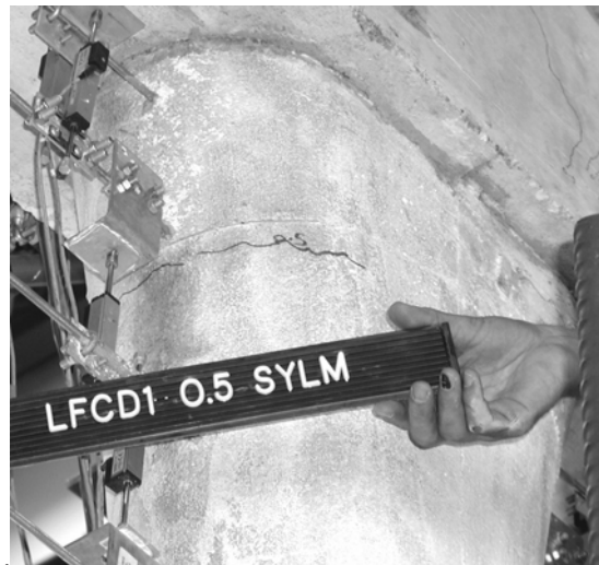
Fig. 4-3 LFCD1 at 0.5 times Sylmar (a) Joint Cracks (b) Flare Cracks
