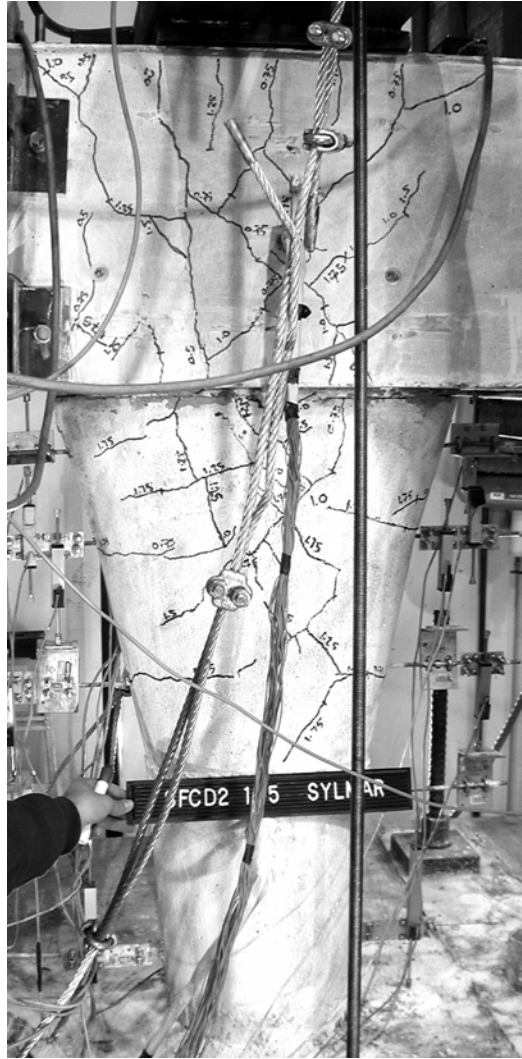
Fig. 4-112 SFCD2 at 1.75 Times Sylmar (a) Column & Joint (b) Joint Crack
