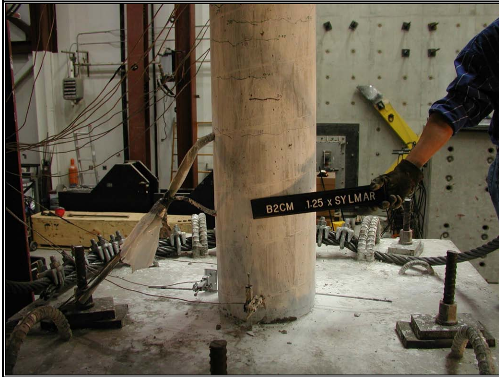
Fig. 4-26: Spalling on West Side of East Column Base
