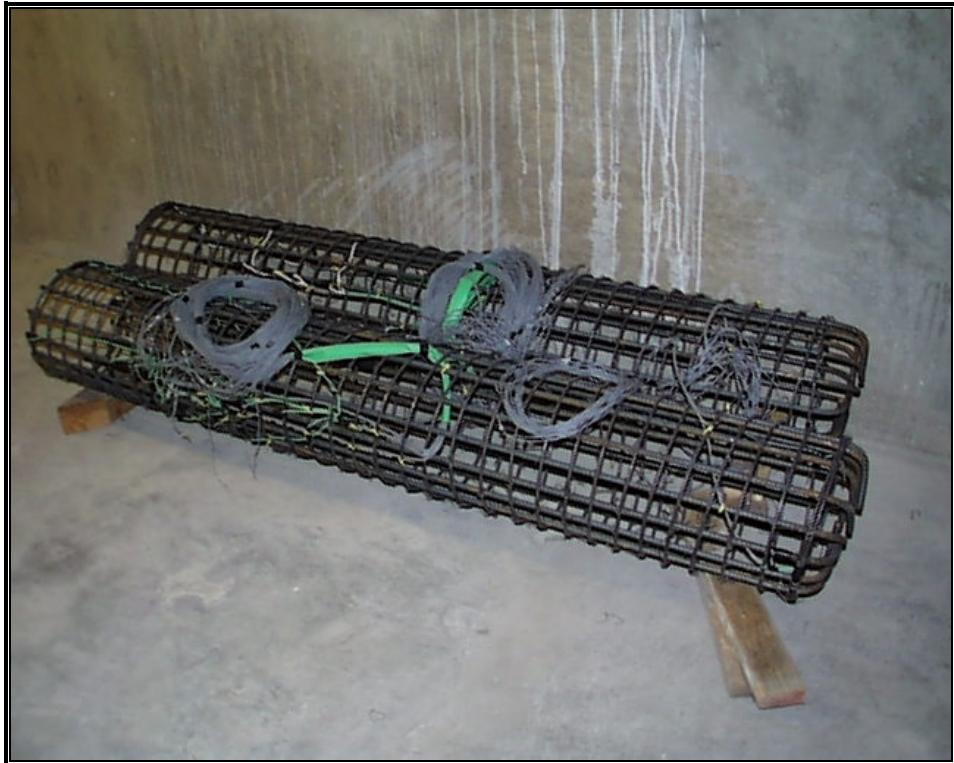
Fig. 3-10: Gaging Process of Medium Specimen Columns
