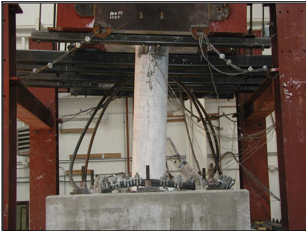
Fig. 4-35: Middle Specimen Leaning after 2.75 x Sylmar
