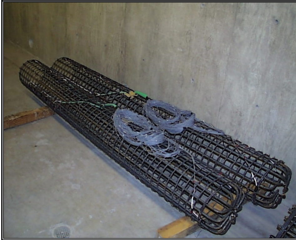
Fig. 3-11: Gaging Process of Tall Specimen Columns
