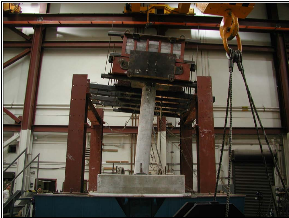
Fig. 4-53: Tall Specimen Leaning after 2.5 X Sylmar
