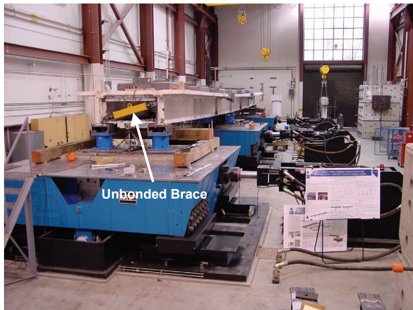
FIGURE 2-3 Testing of Slab-on-Girder Bridge Model with Unbonded Brace End Diaphragm (Adapted from Itani, 2003)
