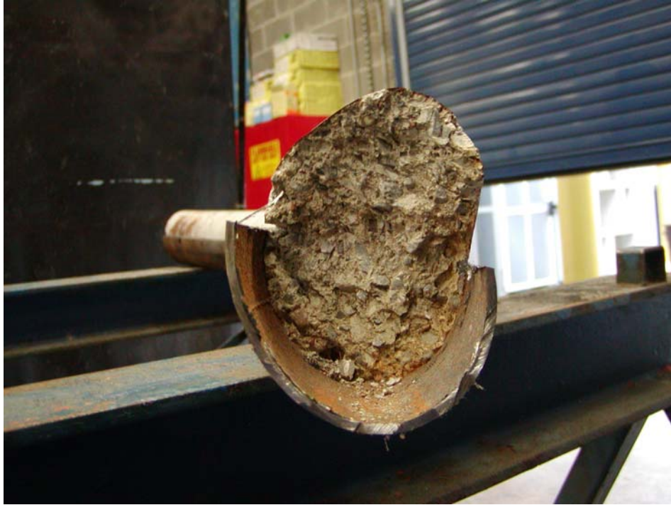
Figure 5-45 Section at Bottom of Column B2-C4 after Test 7
