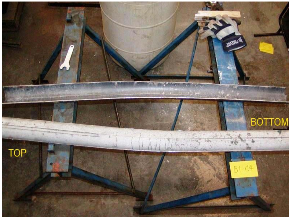
Figure 5-10 Core Concrete of Column B1-C4 after Test 3
