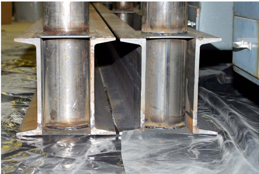
Figure 4-15 Column-to-cap Beam Connection
