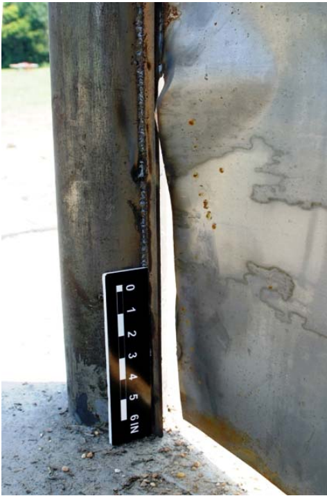
Figure 5-50 Fracture of Plate at C5 Side (Plate B2-SP56 after Test 8)
