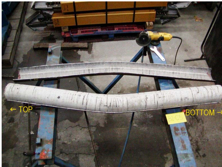
Figure 5-26 Core Concrete of Column B1-C5 after Test 5
