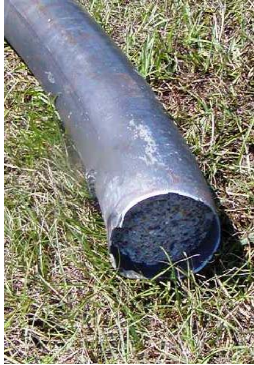
Figure 5-38 Cut Section on Top of Column B2-C4 after Test 7
