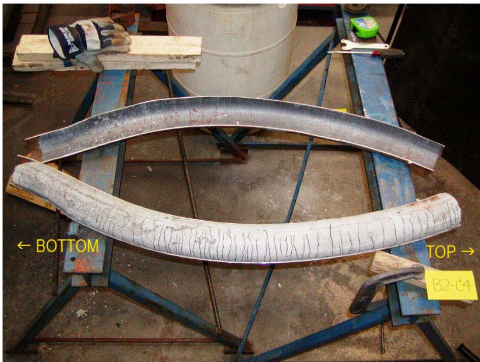
Figure 5-44 Core Concrete of Column B2-C4 after Test 7
