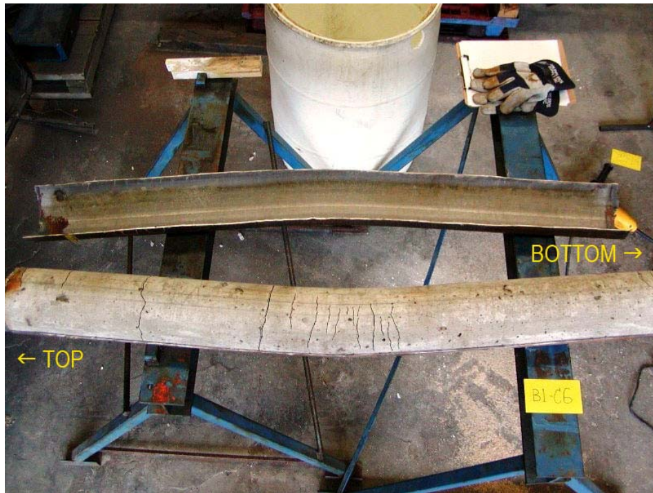
Figure 5-18 Core Concrete of Column B1-C6 after Test 4
