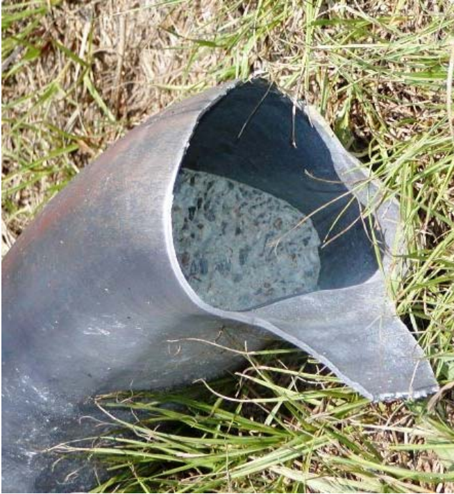
Figure 5-37 Cut Section on Bottom of Column B2-C4 after Test 7
