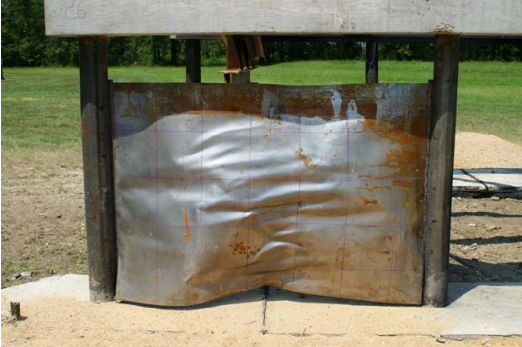
Figure 5-47 Deformation of Plate B2-SP56 after Test 8 (Front Face)
