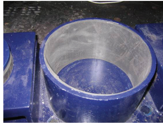
(b) Rubber Strips Rolled inside Pipe to Form Tubular Rubber Pad
