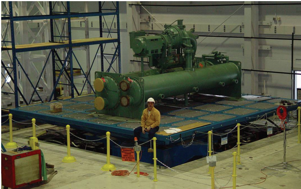
Figure 2-1 Test Specimen: Centrifugal Liquid Chiller
