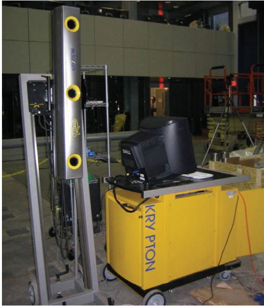
(a) Krypton Coordinate Measurement Machine
