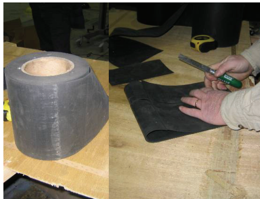
(a) 1.6 mm (1/16 in) Thick Rubber Role (Left) Cut to Strips (Right)
