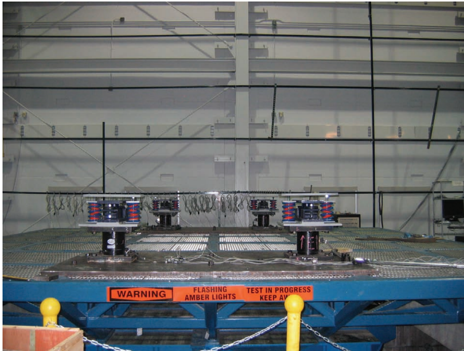
(c) I/R Systems Bolted to Load Cells
