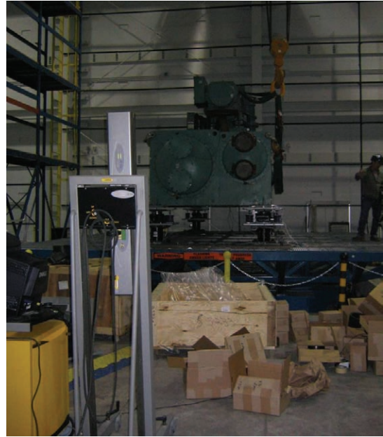
(a) Krypton Coordinate Measurement Machine
