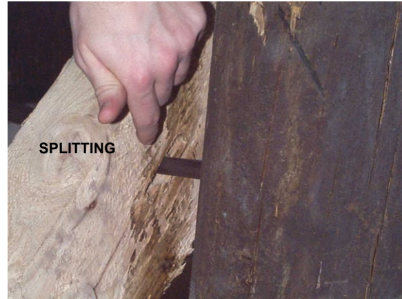
Figure 3-36. Hemlock bracing after test. Photo on left shows minor splintering; photo on right shows splitting in the connection.
