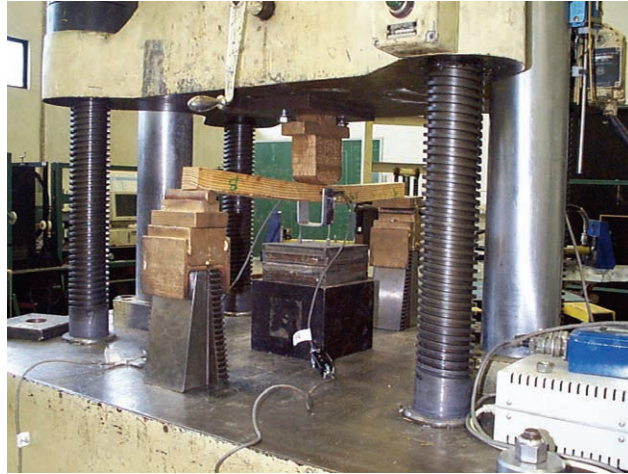
Figure 4-8. Static bending test.
