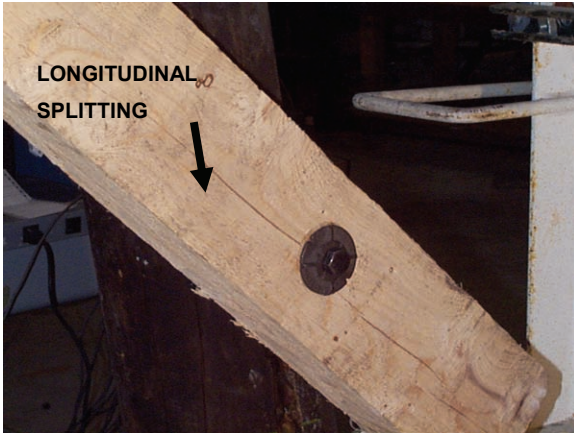
Figure 3-36. Hemlock bracing after test. Photo on left shows minor splintering; photo on right shows splitting in the connection.
