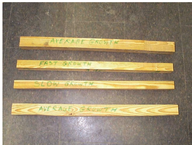
Figure 4-7. Tangential surfaces of bending specimens.
