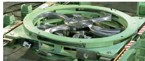
Figure 2-9 Isolation system of the Bolu viaduct 1 (Marioni et al., 2000)
