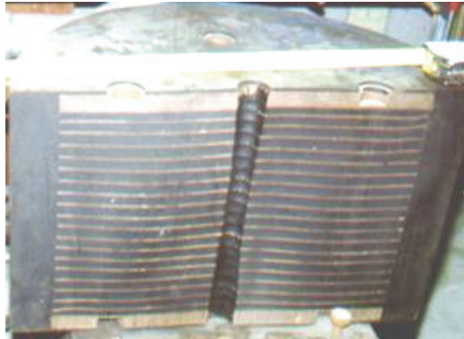
FIGURE 2-10 Section Through an Elastomeric Bearing
