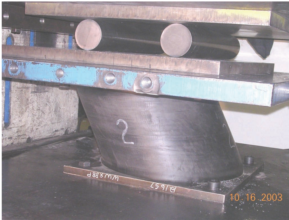
FIGURE 8-14 Lead-Rubber Bearing During High Speed Testing
