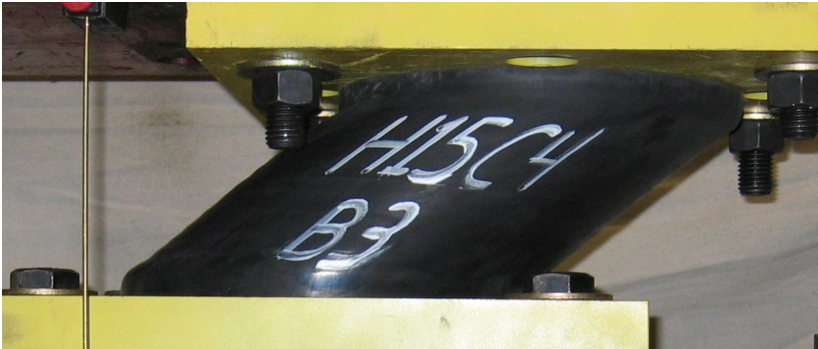
FIGURE 7-8 View of Bearing of Figure 7-7 during Large Lateral Deformation Test
