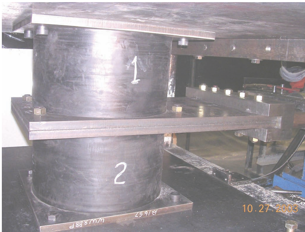
FIGURE 8-15 Lead-Rubber Bearings Tested in Pairs in the 1.6km Cumulative Travel Test
