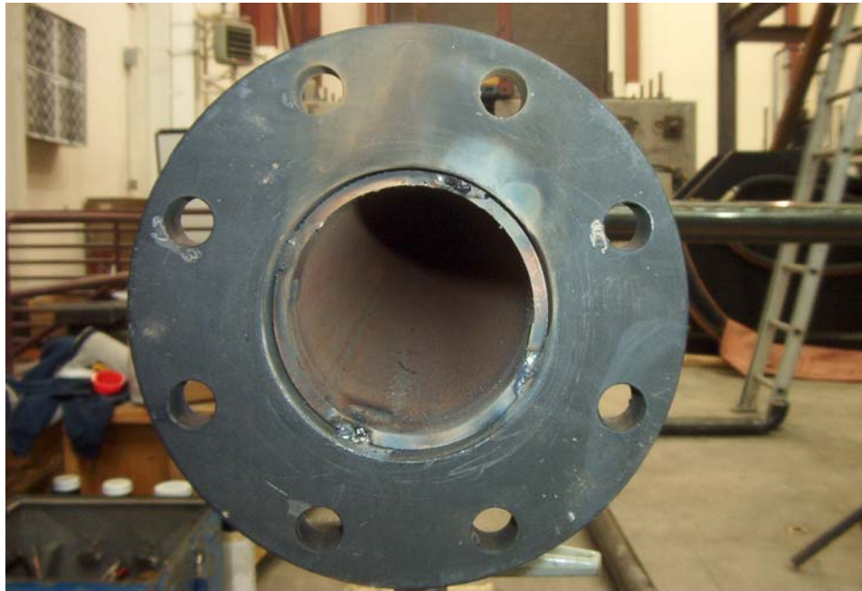
Figure 2-5 Eight Bolt Flanged Connection to Valves and Heat Exchanger
