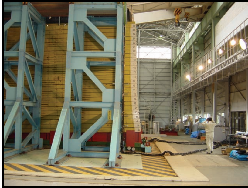
Figure 1.17: Final free field deformation profile of 6 m inclined laminar box after Test No.1, NIED, Japan (Sato et al., 2004, unpublished)
