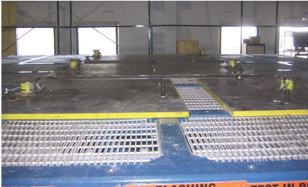
Figure 5-6 Six Load Cells Bolted to Interface Plates
