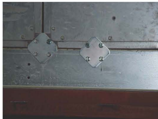
(c) Strengthening of Test Specimen Housing by Additional Connection Plates between Base Rail and Housing
