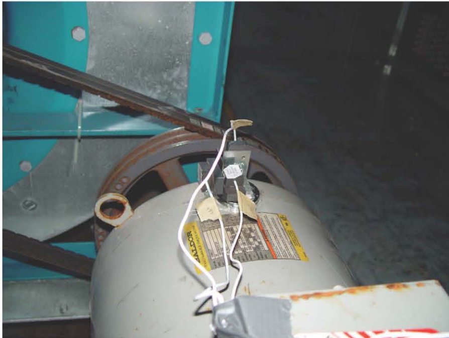
Figure 4-3 Triaxial Accelerometers Installed Close to Center of Mass of Test Specimen, Top of Motor inside Fan Module
