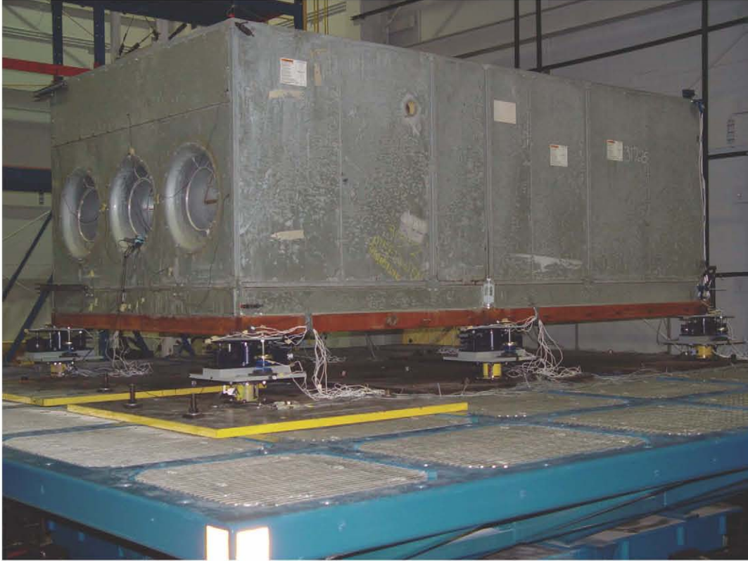
Figure 5-7 Test Setup, Phase I: Test Specimen Mounted on Six I/R Systems
