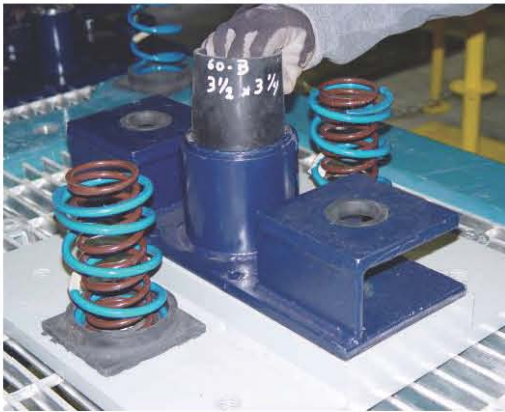
(c) Placing Rubber Tube inside the Bottom Pipe
