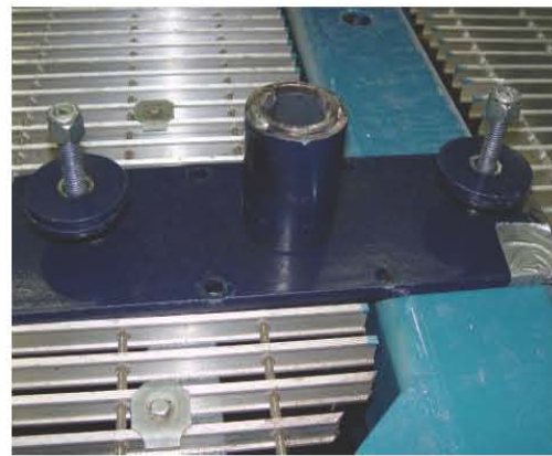
(c) Steel Bushing around Top Pipe to Adjust Horizontal Gap Size
