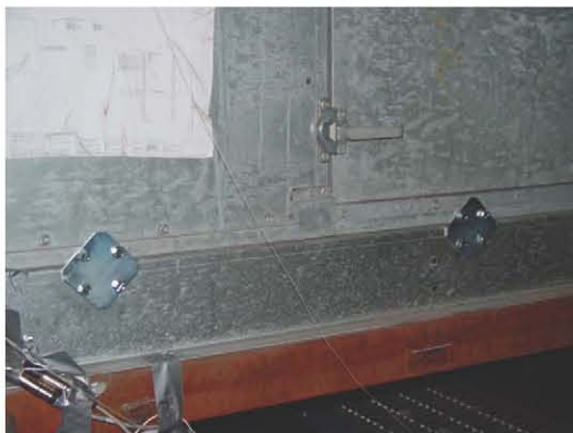
(c) Strengthening of Test Specimen Housing by Additional Connection Plates between Base Rail and Housing
