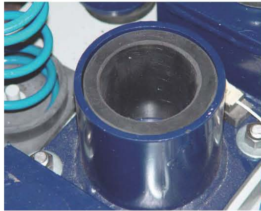
(c) Placing Rubber Tube inside the Bottom Pipe
