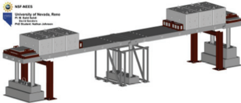
FIGURE 7-1 Experimental Model of a Two-Span Reinforced Concrete Bridge (Johnson et al. 2006)
